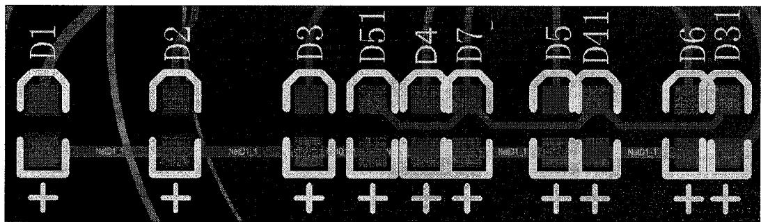
Ten positions of D1, D2, D3, D51, D4, D7, D5, D41, D6 and D31 on PCB board.
