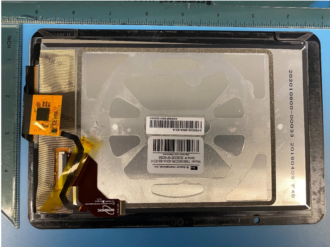
Figure 9: LCD and Touch screen back view
