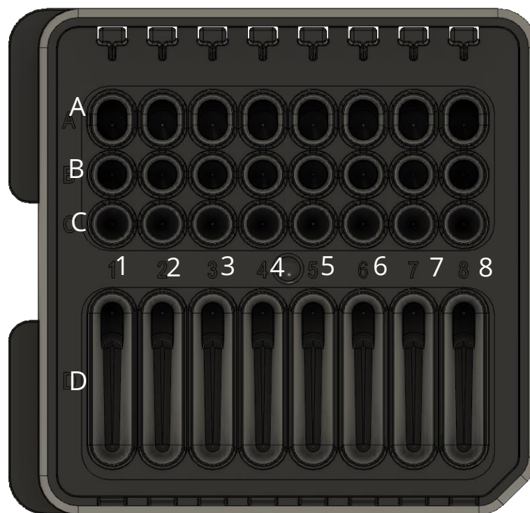
Fig. 2.3 . Top view of Xdrop DE20 Cartridge with the wells (A–D) and lanes (1–8) marked.
