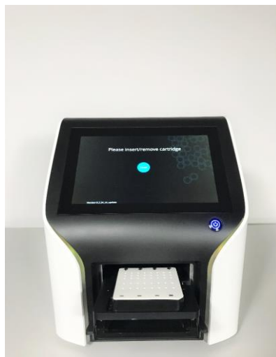
Fig. 3.6. Xdrop Sort with a correctly inserted Xdrop DE20 Sort Cartridge. Position the cartridge correctly to avoid damaging the instrument or cartridge.
