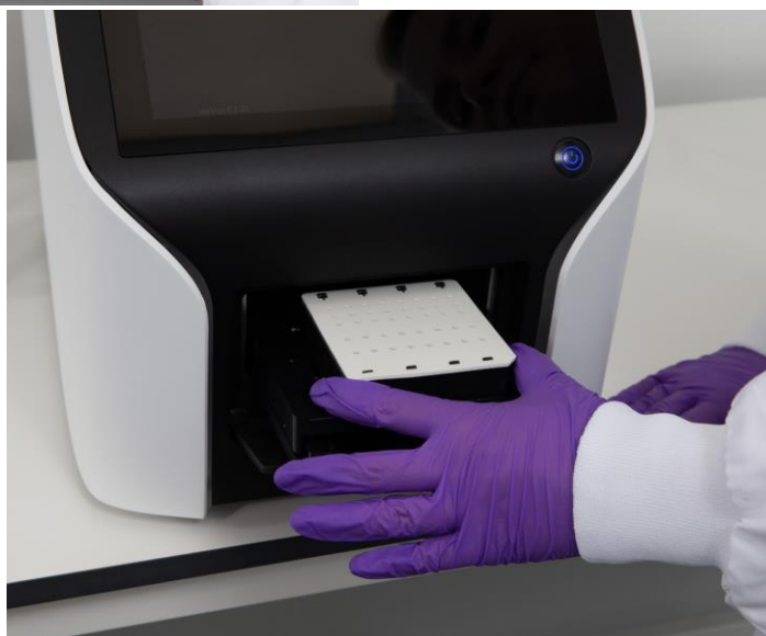
Fig. 2.7. Two views of Xdrop Sort with a correctly inserted Xdrop DE20 Cartridge. Position the cartridge correctly by aligning the angled corner on the cartridge with the angled corner in the drawer. to avoid damaging the instrument or the cartridge.
