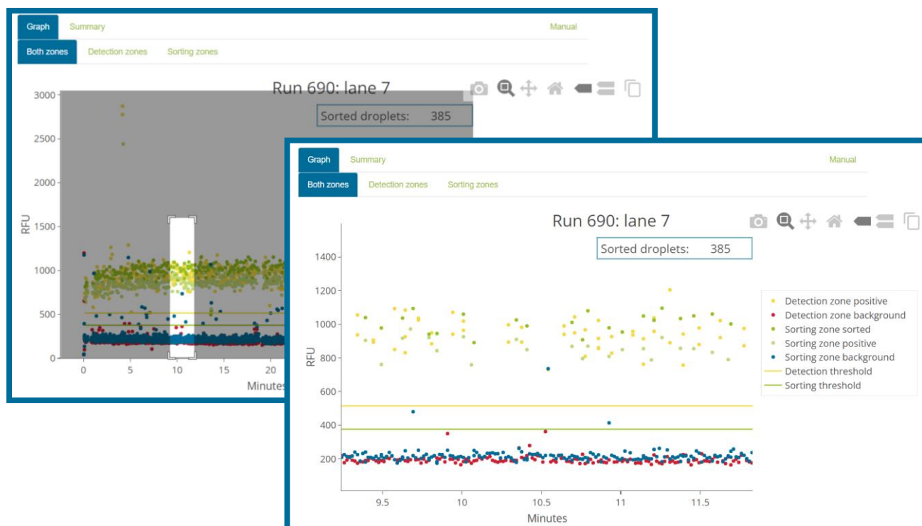
Fig. 4.9. Use the mouse to select an area of the plot to zoom in on. Use the scroll button on your mouse to zoom in and out.
