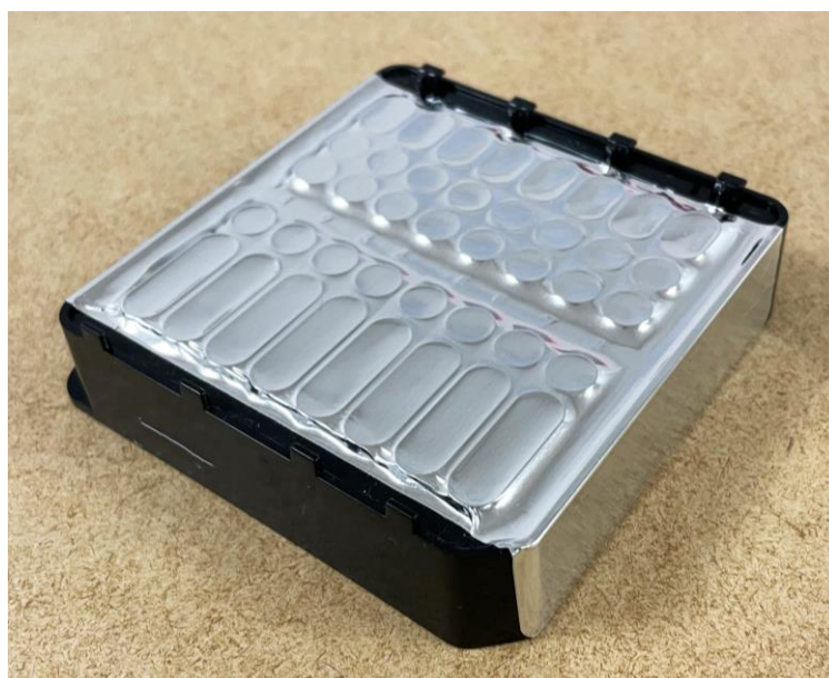
Fig. 3.2. Xdrop DE20 Sort Cartridge sealed with foil for sorting. Make sure to carefully cover all wells.
