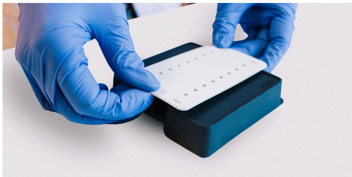
Fig. 5.6. Attach white rubber gasket to the dMDA cartridge. First insert pins and then T-hooks.
