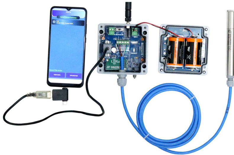
Figure 5-11-1 EWN-01V VW node connected to Android phone with FTDI cable via OTG adaptor
