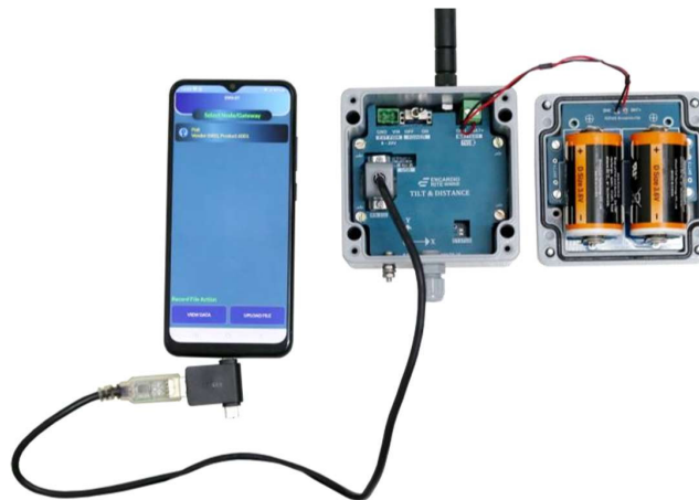
Figure 6-5 NexaWave TiltRange connected to Android phone with FTDI cable via OTG adaptor
