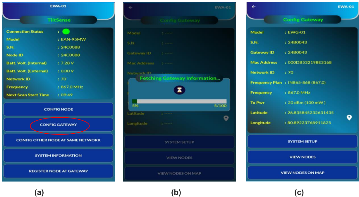
Figure 7-1 Config gateway (via tilt meter node)
