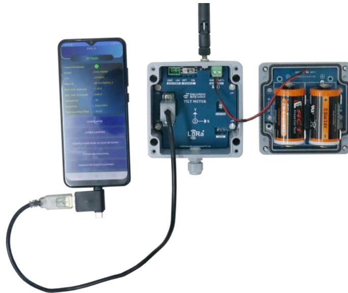
Figure 6-5 Tilt meter connected to Android phone with FTDI cable via OTG adaptor
