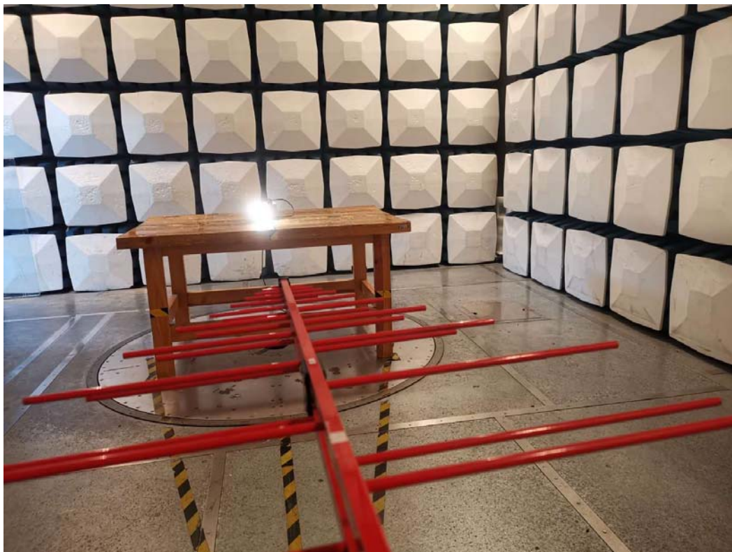
Radiated Emission Above 1GHz View
