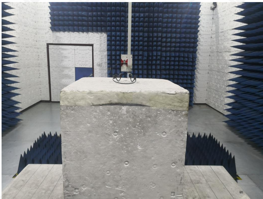
RADIATED EMISSION TEST SETUP ABOVE 1GHZ
