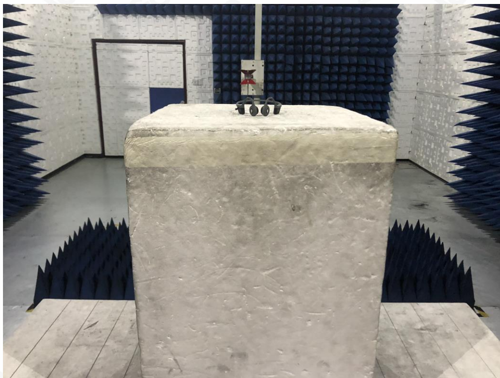
RADIATED EMISSION TEST SETUP ABOVE 1GHZ
