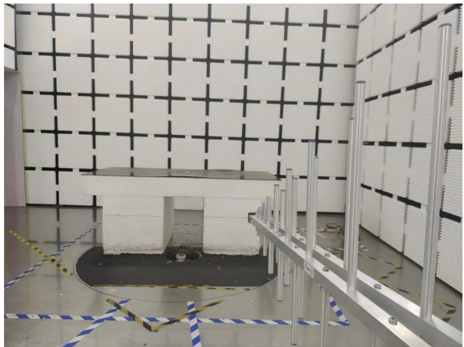
Radiation Emission Test Setup (30MHz to 1GHz)
