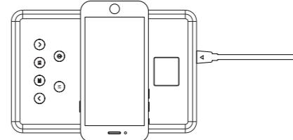
4. When using the line charger, insert one end of the USB charging cable into the USB port at the end of the desk lamp, and connect the other end to the mobile phone. (As shown below)
