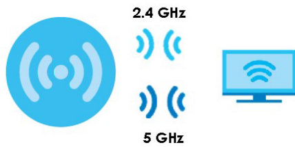
Figure 103 Multi-Link Operation Example
