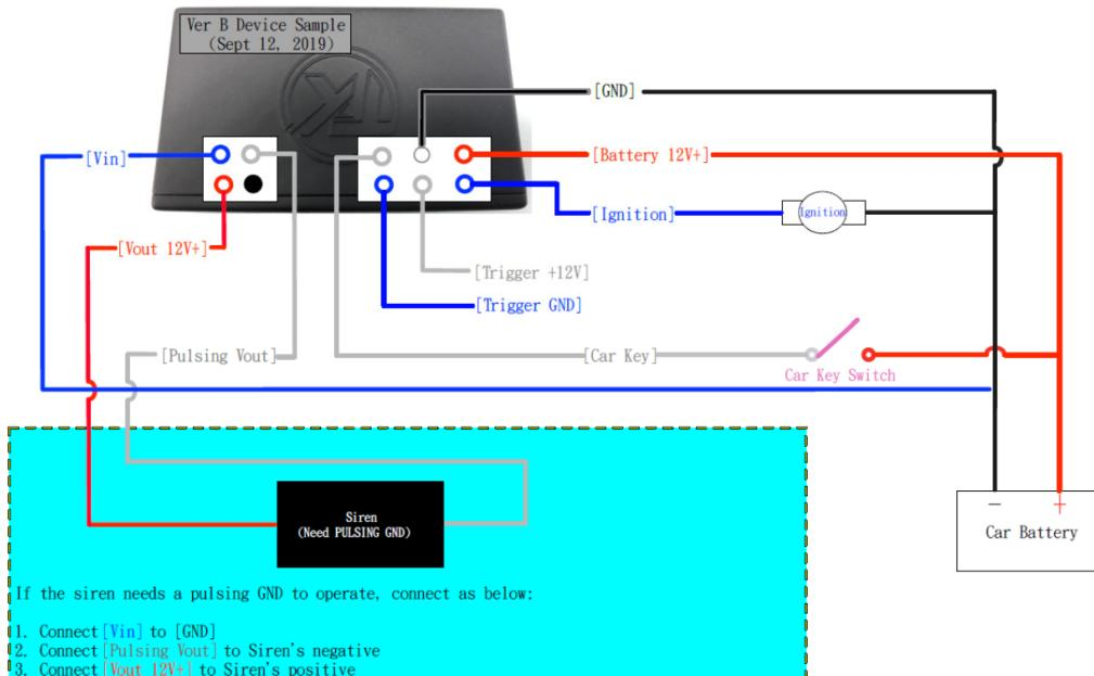
*Note: You may connect [Trigger +12V] and/or [Trigger GND] to any device to activate the receiver, such as pin-switch, door or any sensor from the car.*
