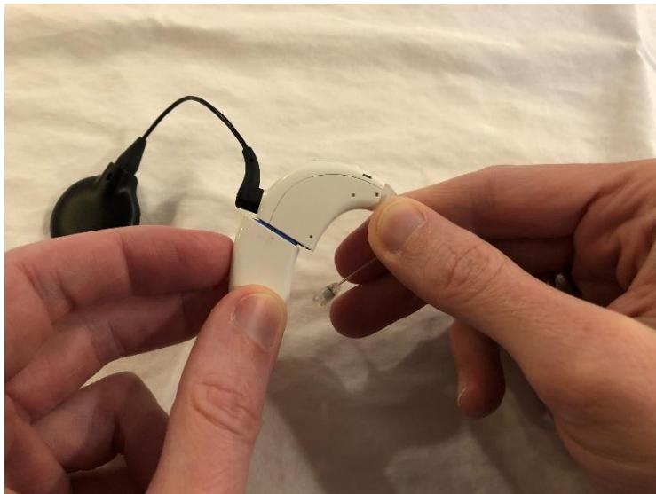
Continue sliding the battery until it separates from the sound processor.
