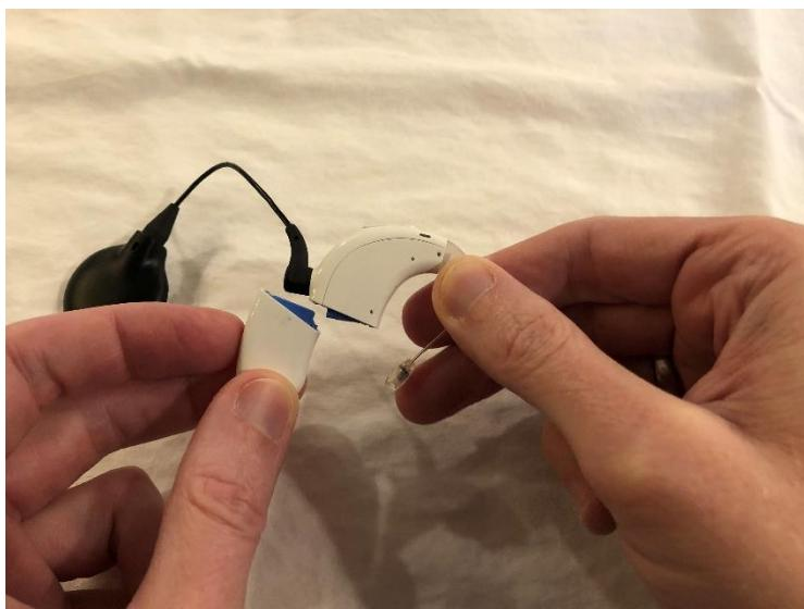
Align the battery connector with the sound processor housing side of the connector.
