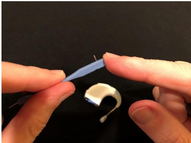
Line up the pin with the hole in the earhook and gently push it through the hole. The pin will move from one side of the sound processor, through the earhook to the other side of the sound processor, holding the earhook in place. The pin should not come out the other side.
