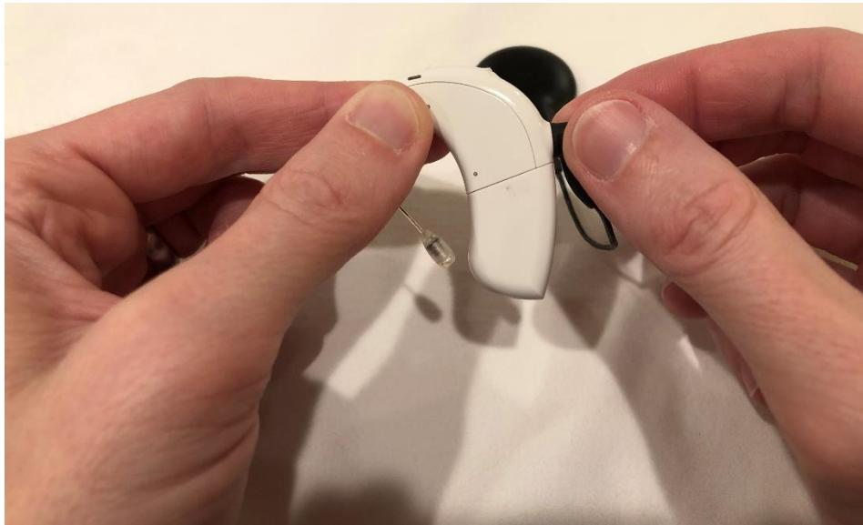
NOTE: To maximize cable life, the cable should only be unplugged from the sound processor when changing wearing configuration or when replacing the cable.
