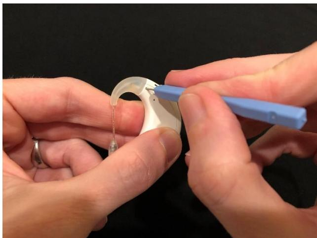
Gently press the tool in the hole, pushing the pin out the other side.
