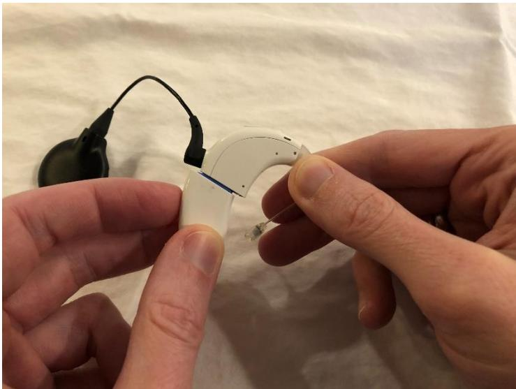
Slide the battery onto the sound processor until it clicks into place. Do not force the battery onto the sound processor. The batteries are designed to be inserted in only one direction; applying force may damage the equipment.
