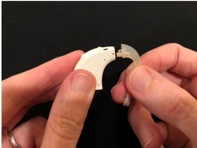
Using the provided pin removal tool, place one of the pins in the small hole on the side of the tool. This will help to steady the pin as you line it up with the pin hole on the earhook.
