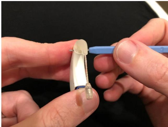
The pin does not need to be removed from the sound processor. As long as the tool is pushed in flush on one side of the sound processor, the pin should be displaced enough to adequately remove the earhook. Remove the tool from the sound processor. Gently grasp the earhook at the top near where it connects with the sound processor and pull forward until it is separated from the sound processor.
