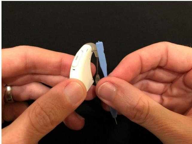
If a small portion of the pin extends beyond the sound processor, use the side of the tool to push the pin inwards so it lies flush with the sound processor.
