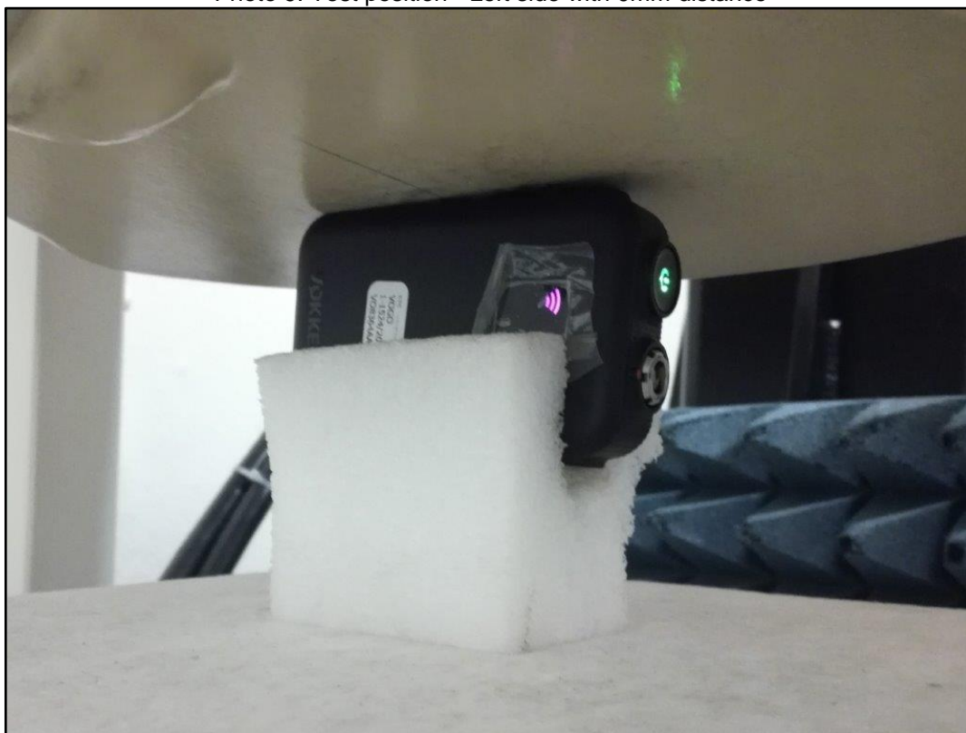
Photo 10: Test position - Right side with 0mm distance
