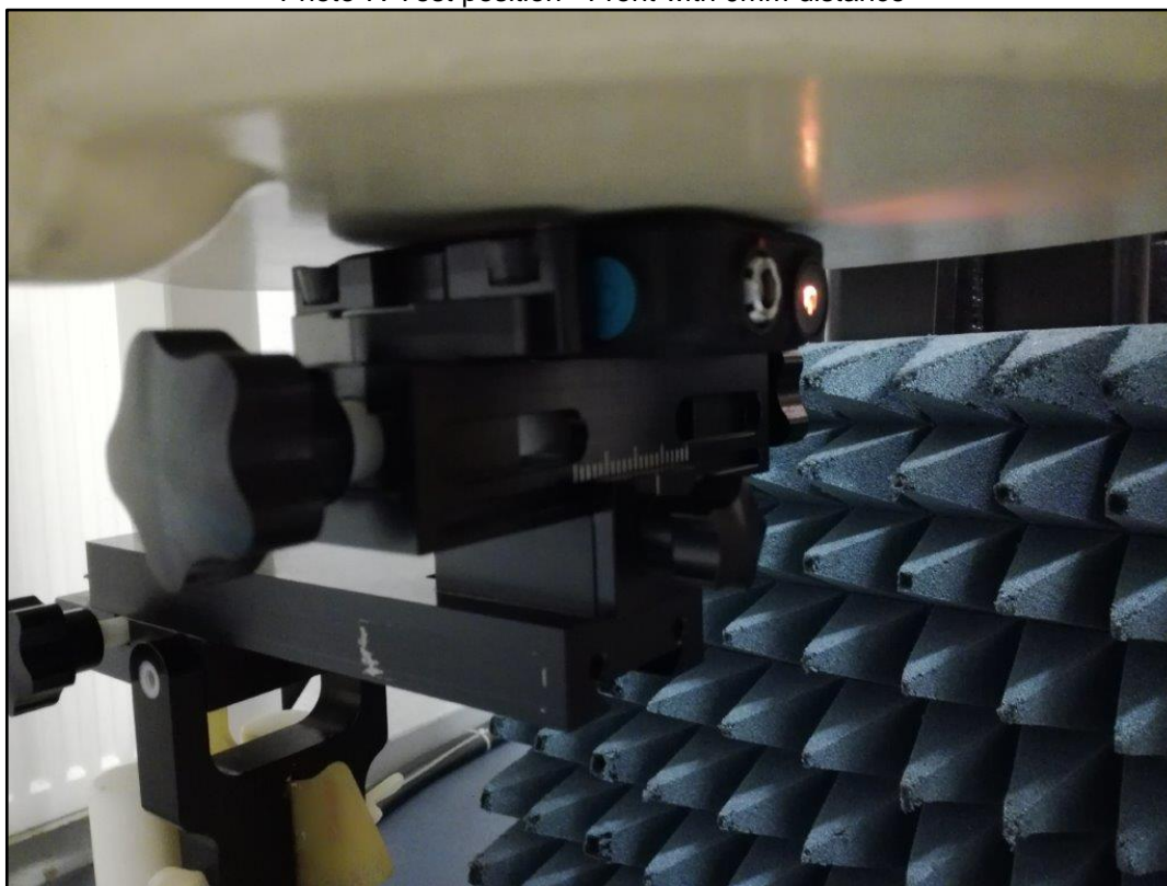
Photo 8: Test position - Rear with 0mm distance
