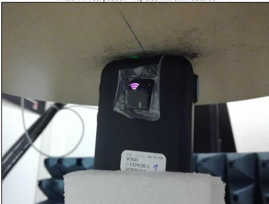
Photo 12: Test position - Bottom side with 0mm distance
