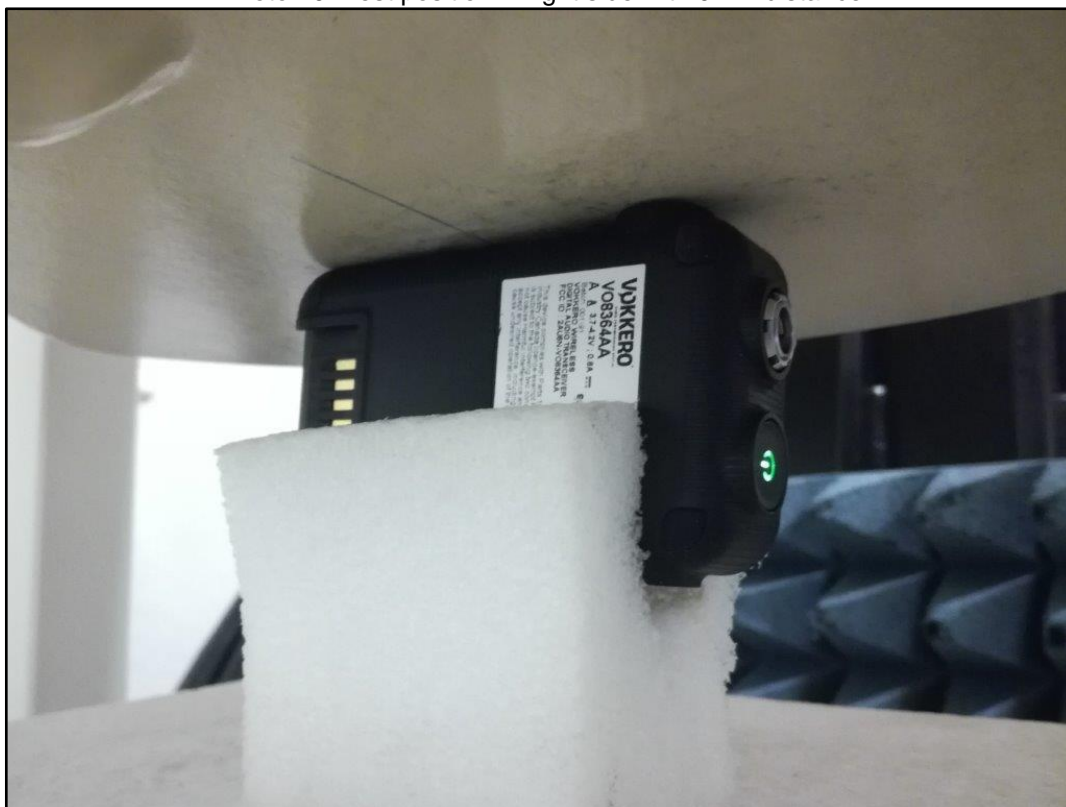
Photo 10: Test position - Right side with 0mm distance
