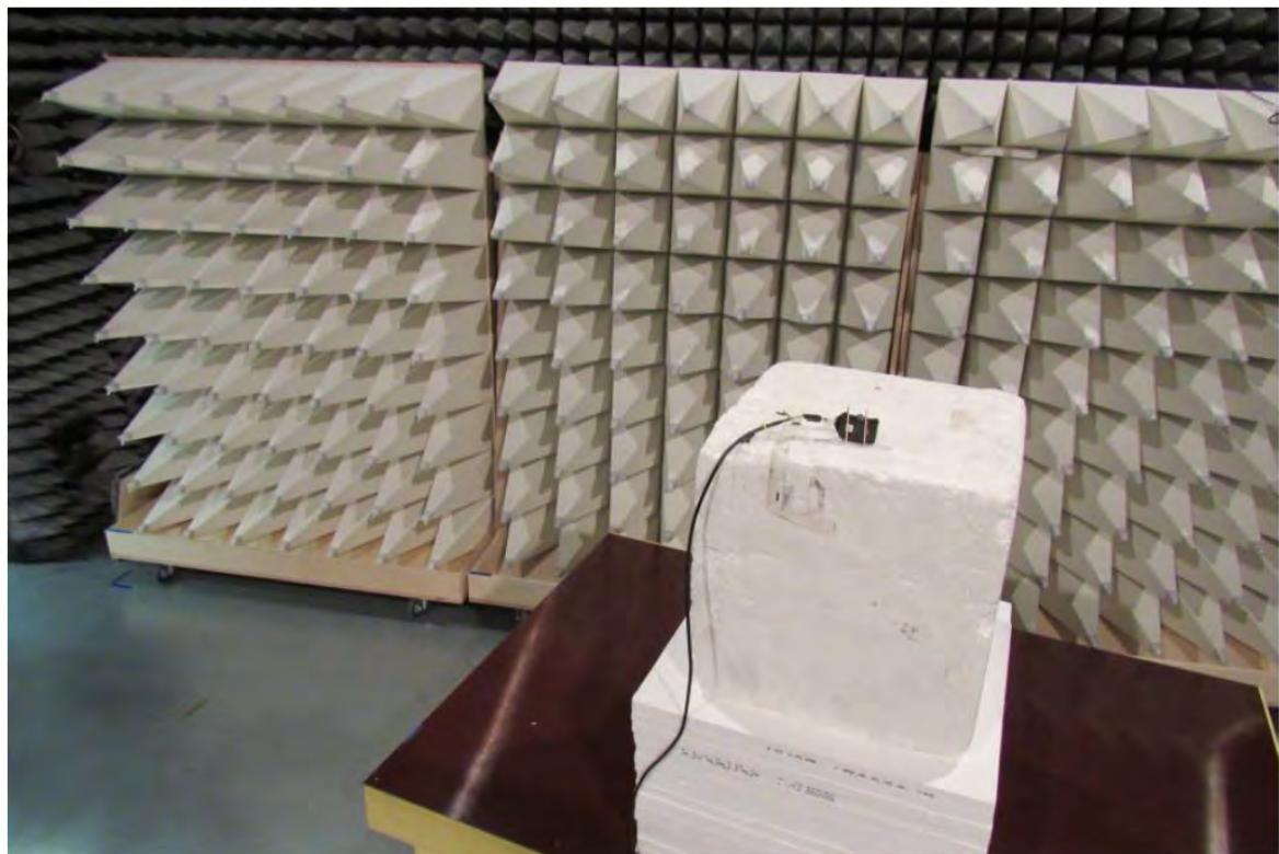
Testsetup EUT view above 1 GHz
