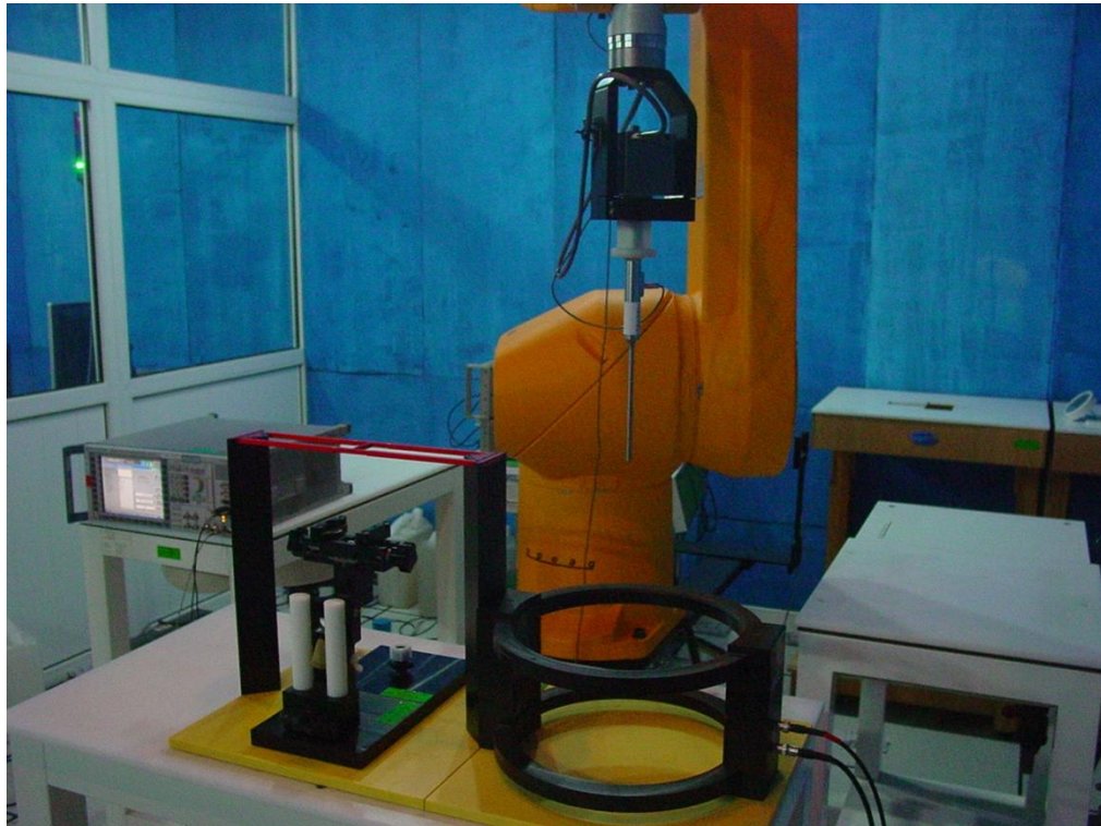
Picture A1: HAC T-Coil System Layout
