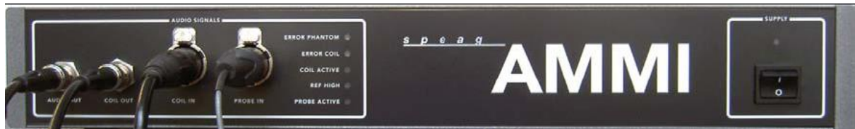
Figure 5.3 AMMI front panel
