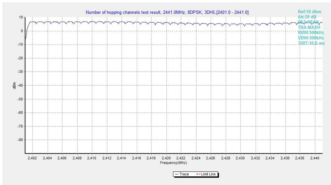
Fig.98. Number of hopping frequencies: 8DPSK, Channel 0 - 39
