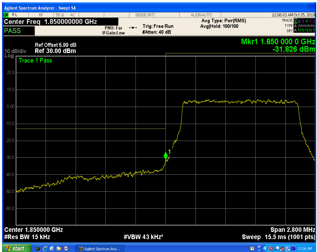
LTE Band2 QAM16 BW=1.4MHz Channel=18607 RB Size=1 Position=#0
