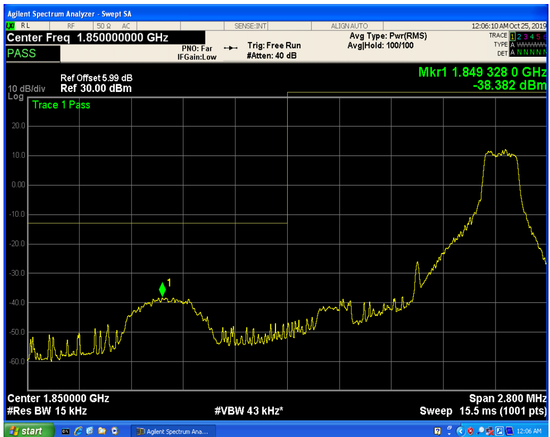
LTE Band2 QAM16 BW=1.4MHz Channel=18607 RB Size=6 Position=#0
