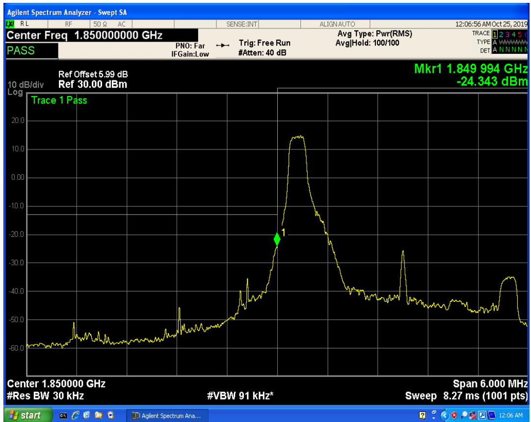
LTE Band2 QPSK BW=3MHz Channel=18615 RB Size=15 Position=#0
