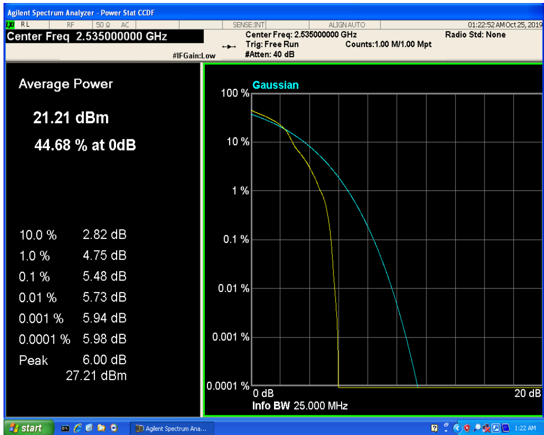
LTE Band7 QPSK BW=15MHz Channel=21100 RB Size=1 Position=#0
