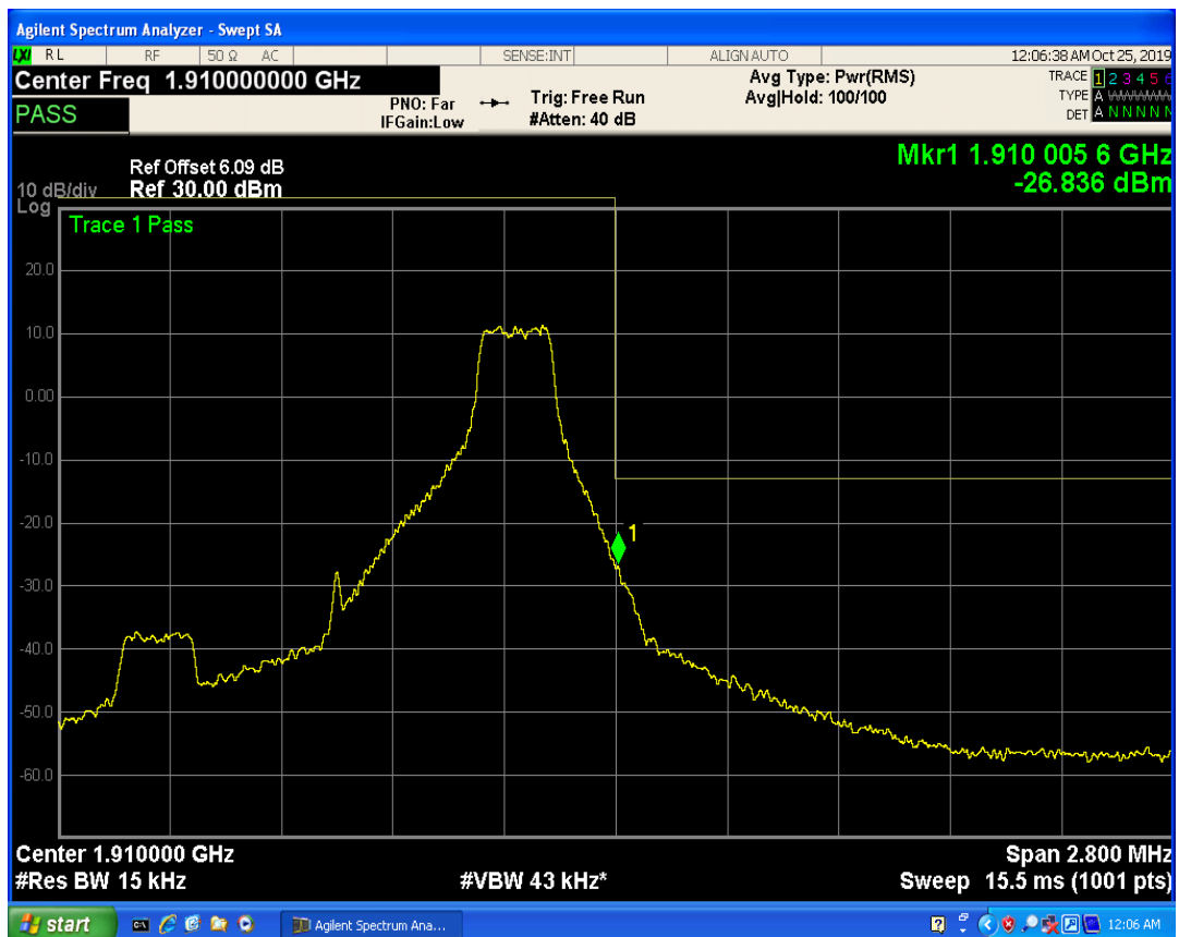
LTE Band2 QAM16 BW=1.4MHz Channel=19193 RB Size=6 Position=#0
