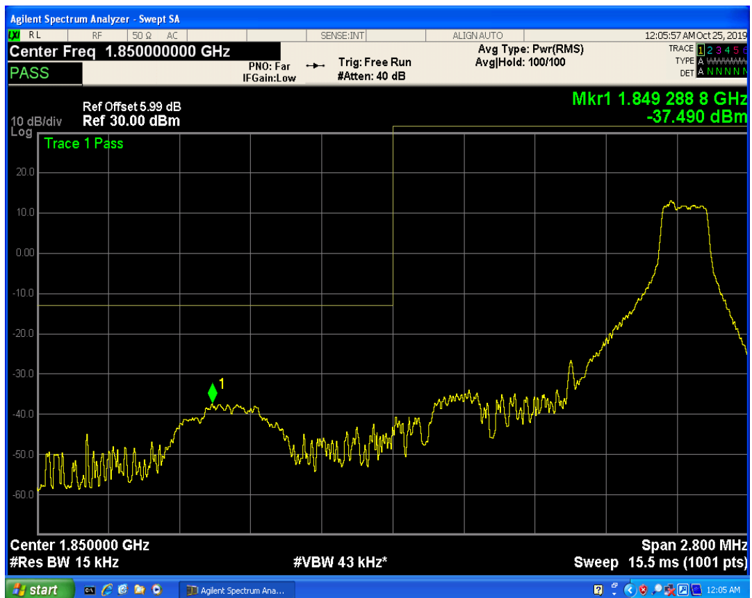
LTE Band2 QPSK BW=1.4MHz Channel=18607 RB Size=6 Position=#0
