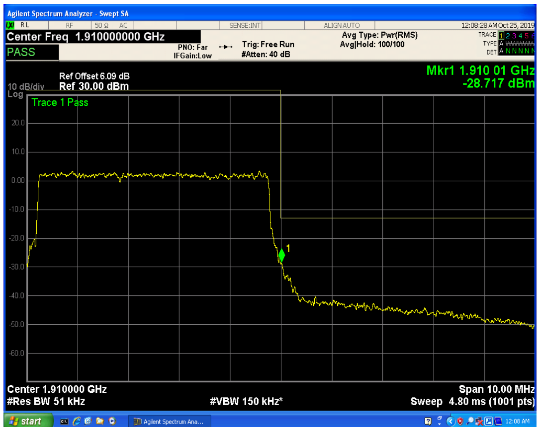
LTE Band2 QAM16 BW=5MHz Channel=19175 RB Size=1 Position=#0
