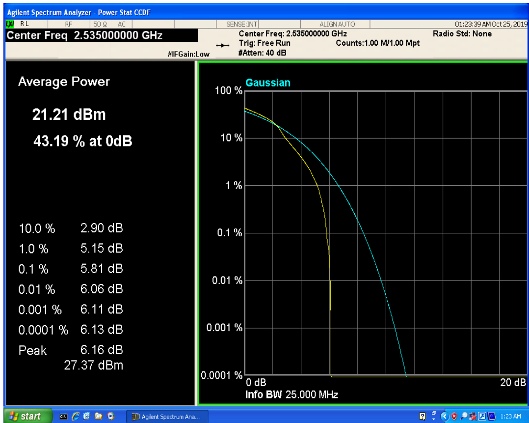
LTE Band7 QPSK BW=20MHz Channel=21100 RB Size=1 Position=#0
