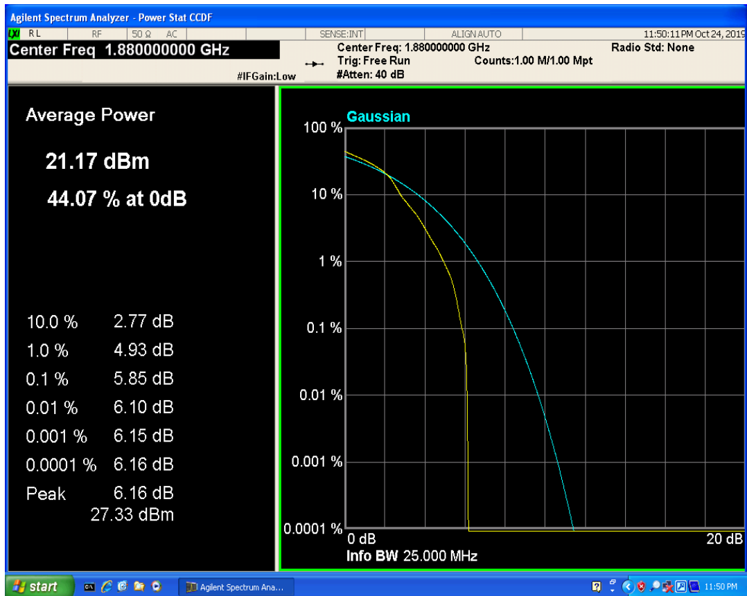
LTE Band2 QPSK BW=15MHz Channel=18900 RB Size=1 Position=#0
