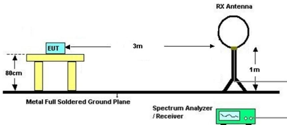
For radiated emissions from 30MHz to 1GHz
