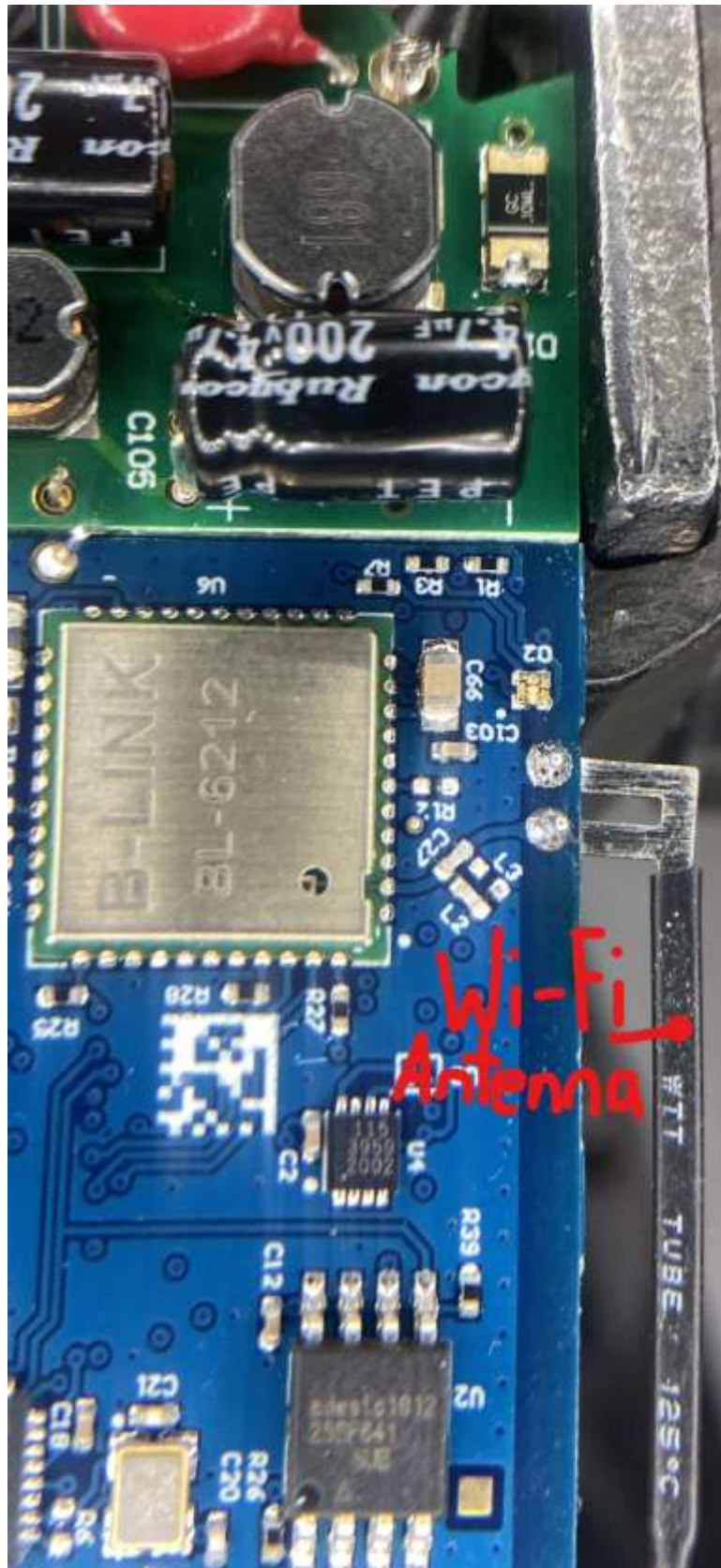
Figure 3: WNRH1 Wi-Fi Antenna
