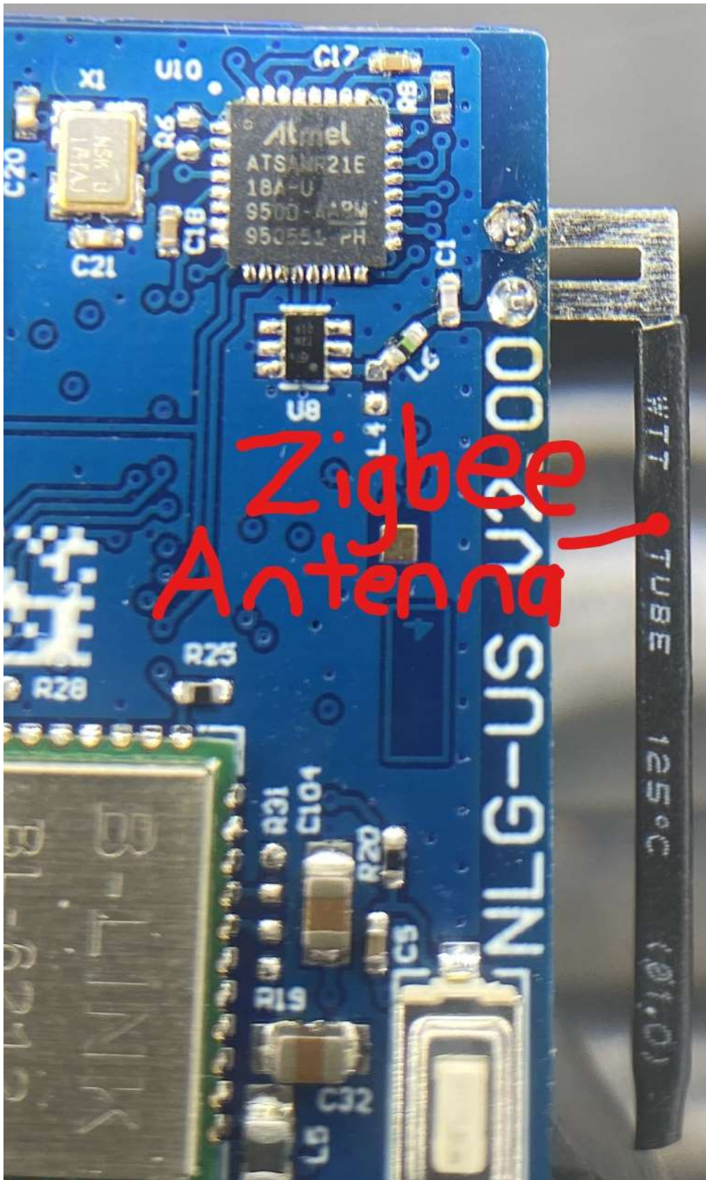
Figure 4: WNRH1 Zigbee Antenna
