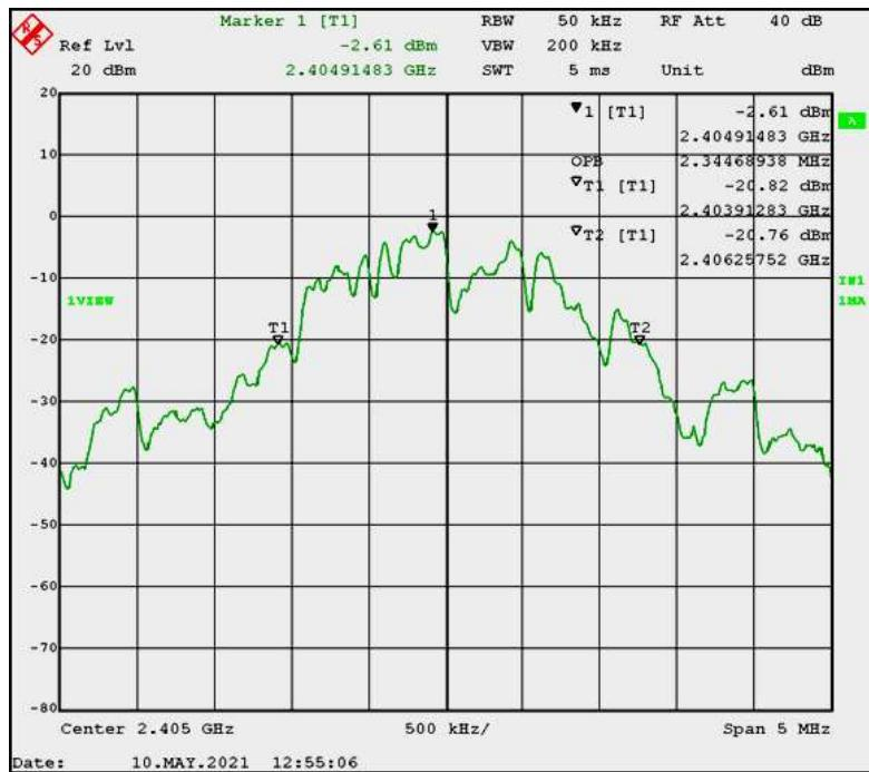
Legrand WNAL43 Zigbee Radio Mid channel 18, 2440 MHz, O-QPSK Modulation
