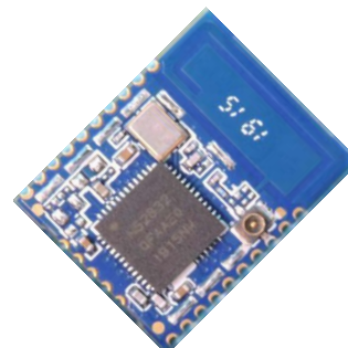
Figure 1: FTK369 Without Shielding Top View protocol stack
