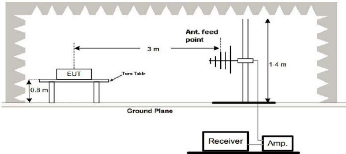
(3) Radiated Emission Test-Up Frequency Above 1GHz
