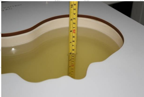
Liquid depth in the Head Phantom (1750MHz)
