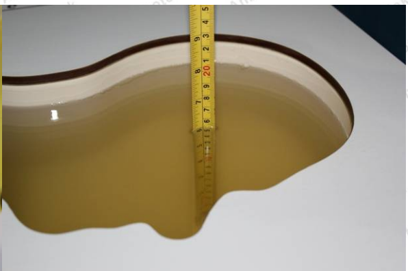
Liquid depth in the Head Phantom (2600MHz)
