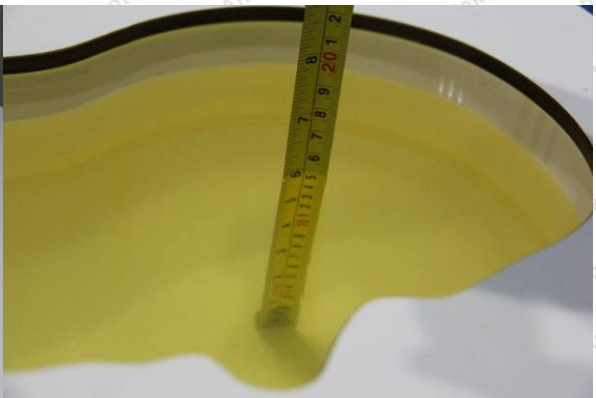
Liquid depth in the Head Phantom (1900MHz)
