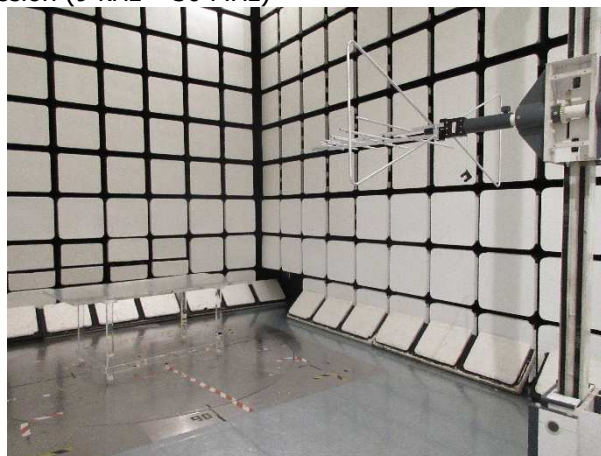
Unwanted Radiated Emission and Unwanted emissions into non-Restricted Frequency Bands (30 MHz – 1 GHz)
