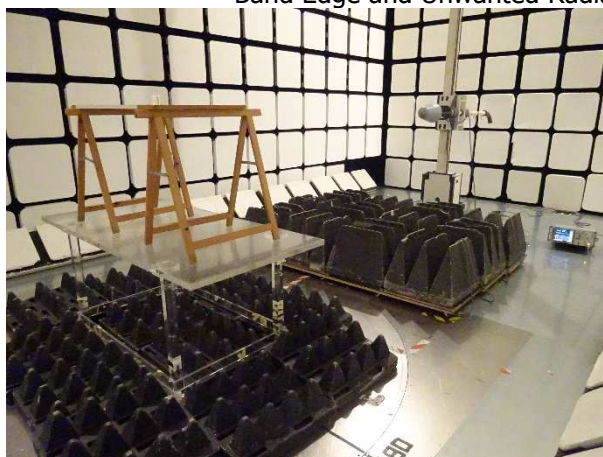
Unwanted emissions into non-Restricted Frequency Bands (1 GHz – 25 GHz) and Unwanted Radiated Emission (18 GHz – 26 GHz)
