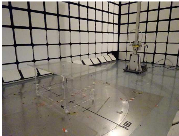
Unwanted Radiated Emission (9 kHz – 30 MHz)
