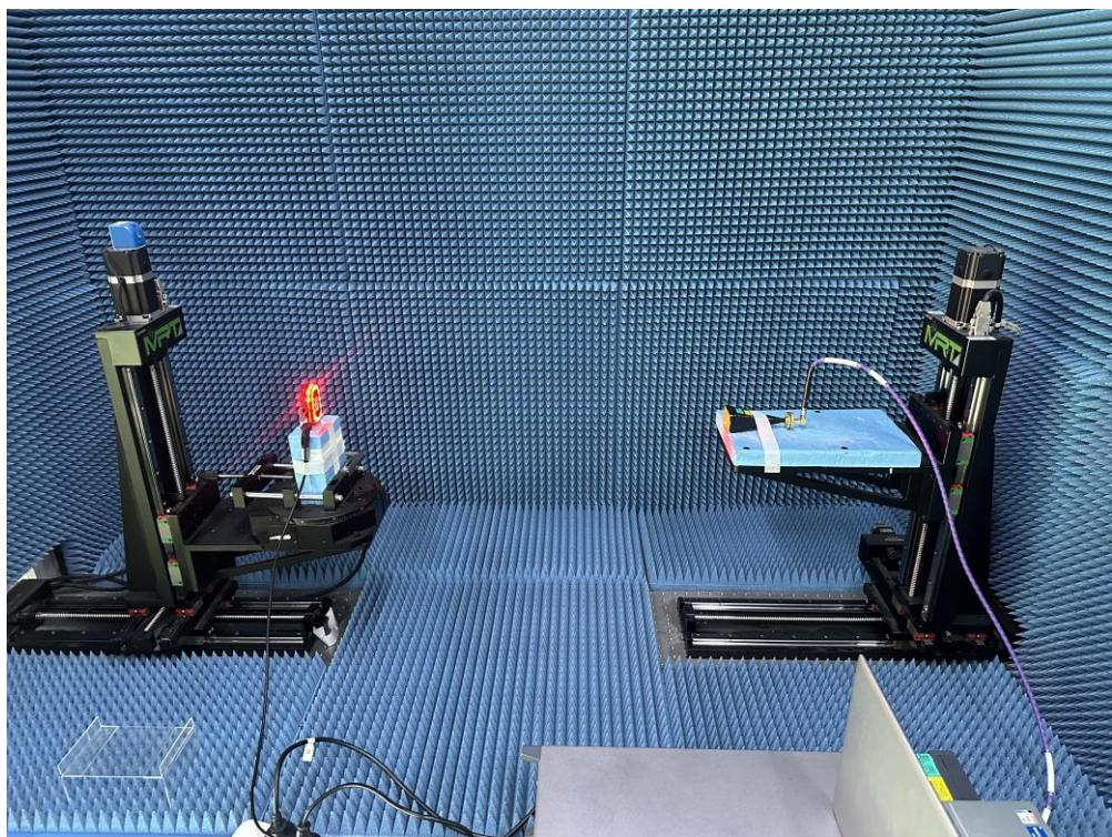
Description: Radiated Spurious Emission Test Setup for 50GHz ~ 75GHz
