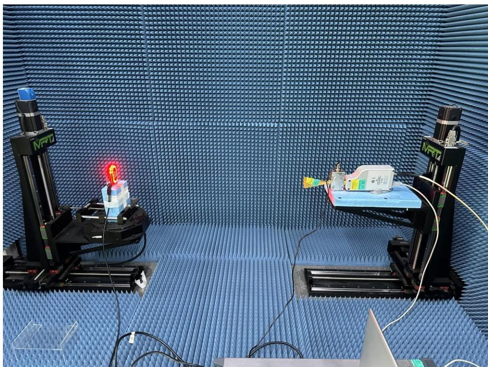
Description: Radiated Spurious Emission Test Setup for 75GHz ~ 100GHz
