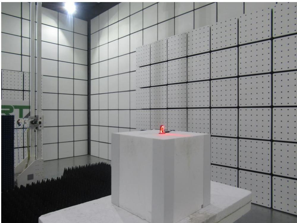
Description: Radiated Spurious Emission Test Setup for 40GHz ~ 50GHz
