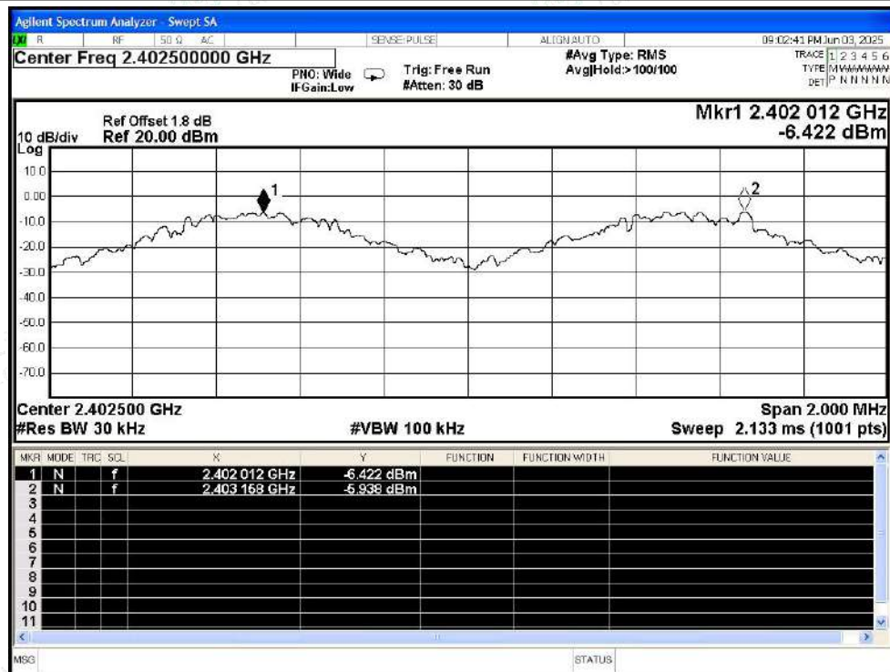
CFS NVNT 2-DH5 2402MHz Ant1
