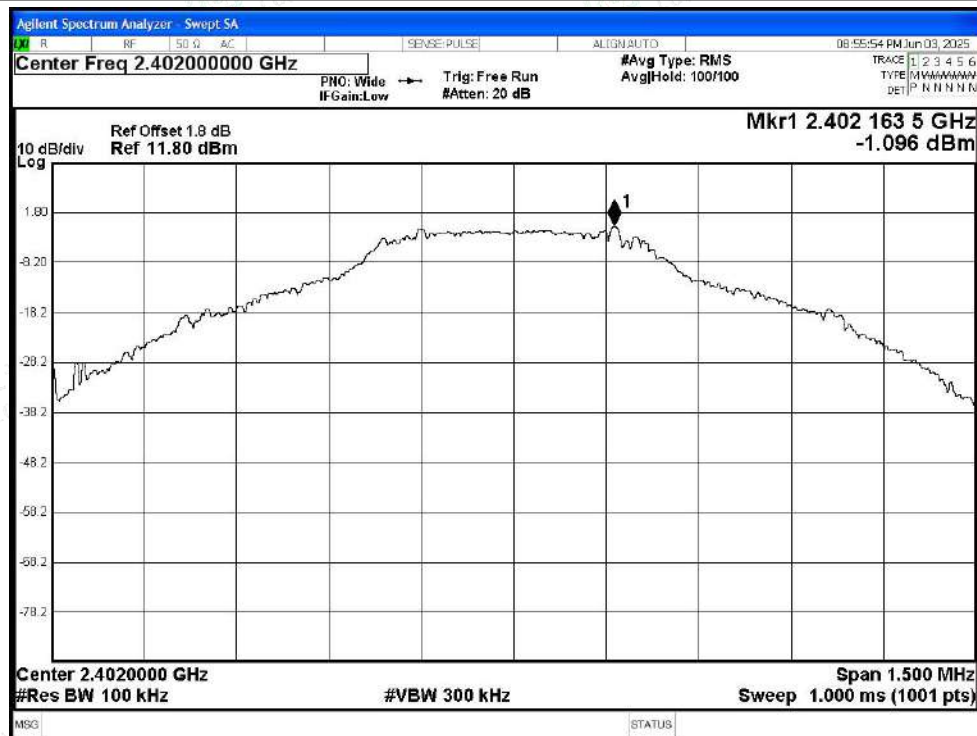
Tx. Spurious NVNT 1-DH5 2402MHz Ant1 Emission
