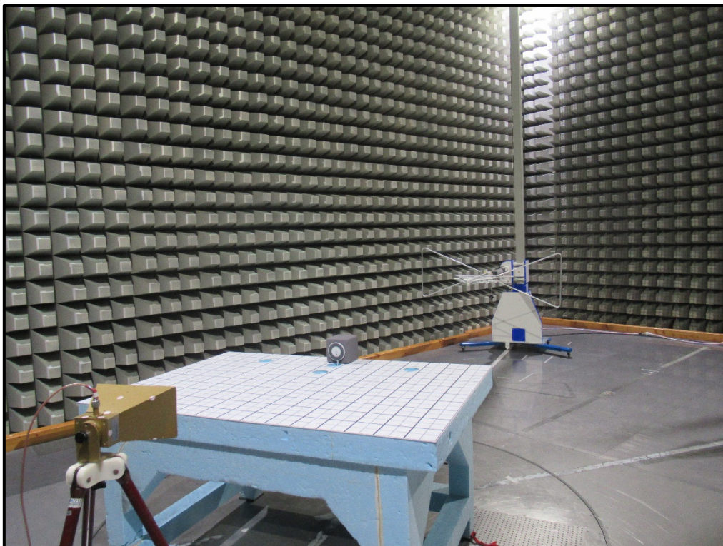
Photo 4 Radiated Test Setup-30 MHz – 1 GHz
