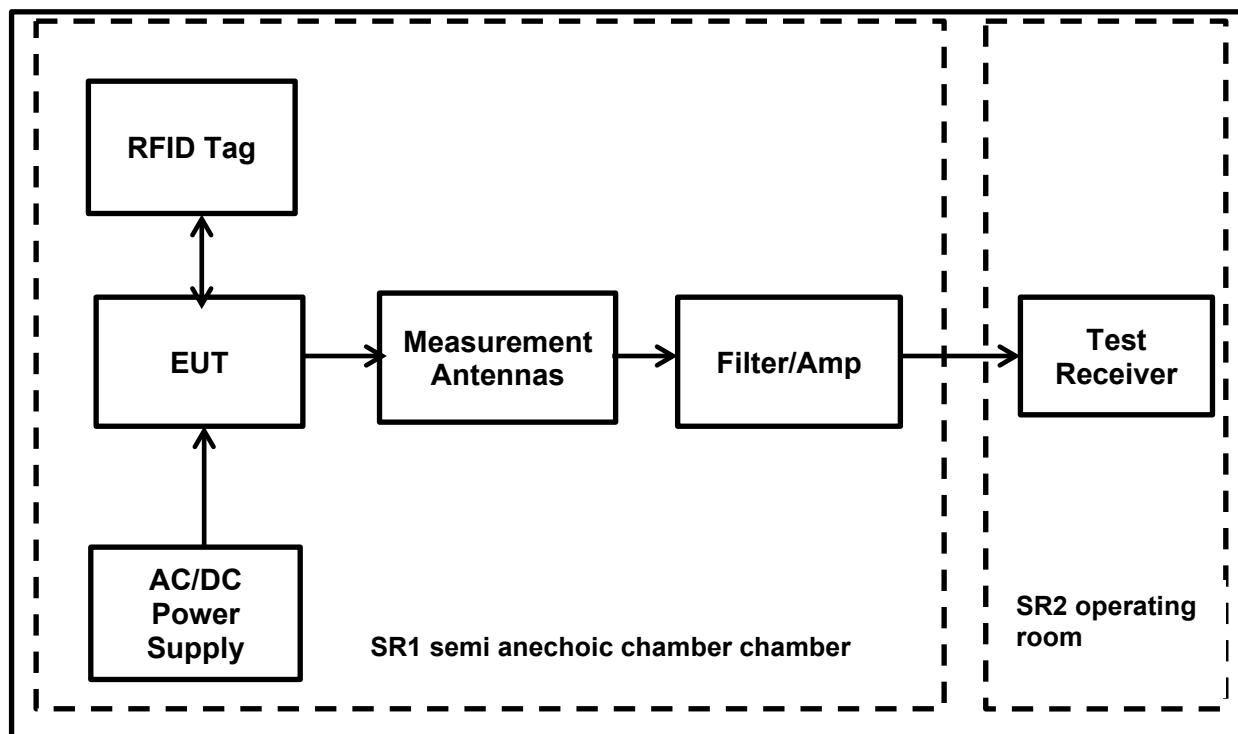
**Transmitter Radiated Emissions (continued)****Results: WLAN 5 GHz / 802.11a / 54 Mbps / PWR 0 / Top Channel + RFID 13.56 MHz**
