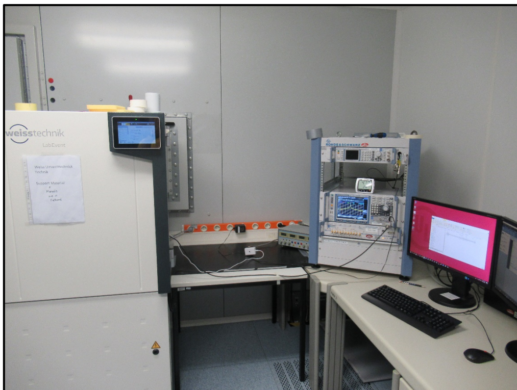
Photo 8 Conducted Test Setup-Frequency Stability
