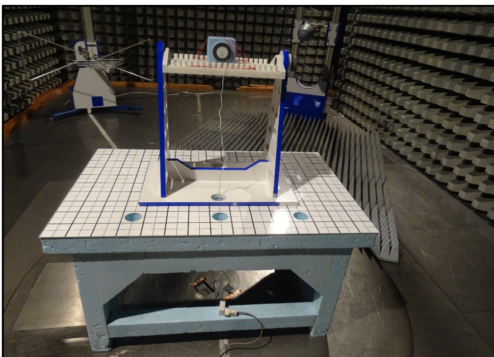
Photo 6: Radiated Test Setup-1 GHz to 18 GHz- with AC/DC Adapter
