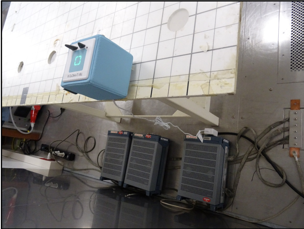
Photo 13 AC Conducted Emissions Test Setup- with AC/DC Adapter
