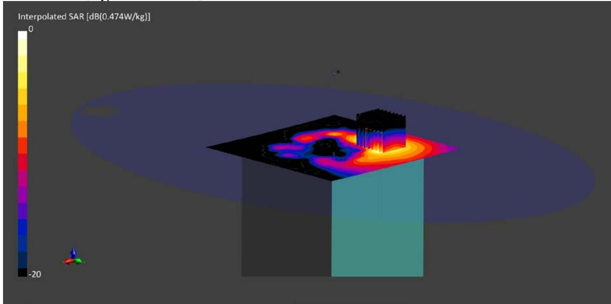
Communication System: IEEE 802.11b WiFi 2.4 GHz (DSSS, 11 Mbps, 99pc duty cycle) UID: 10517; Frequency: 2442.0 MHz; Duty Cycle: 0.99;
