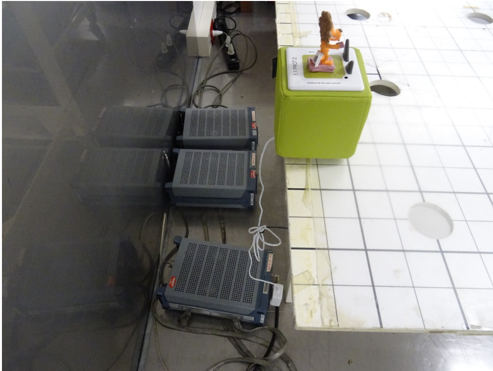
Photo 9: AC Conducted Emissions Test Setup- with AC/DC Adapter
