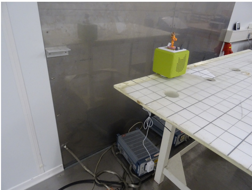
Photo 10: AC Conducted Emissions Test Setup- with AC/DC Adapter
