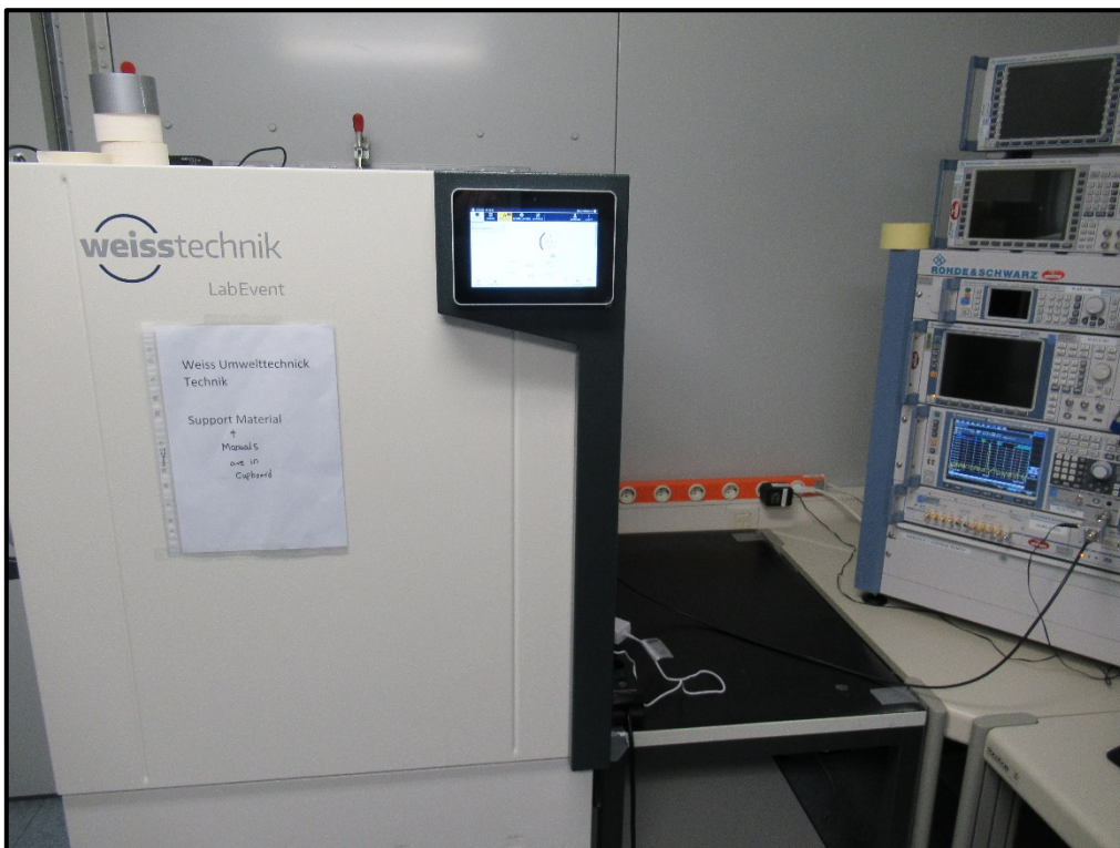
Photo 8: Frequency Stability Test Setup- with Fully Charged Internal Battery
