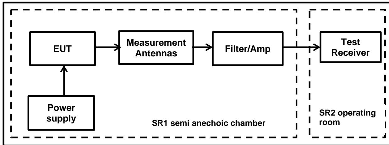
**Transmitter Radiated Emissions (continued)****Results: AC-DC Power supply / RFID 13.56 MHz**
