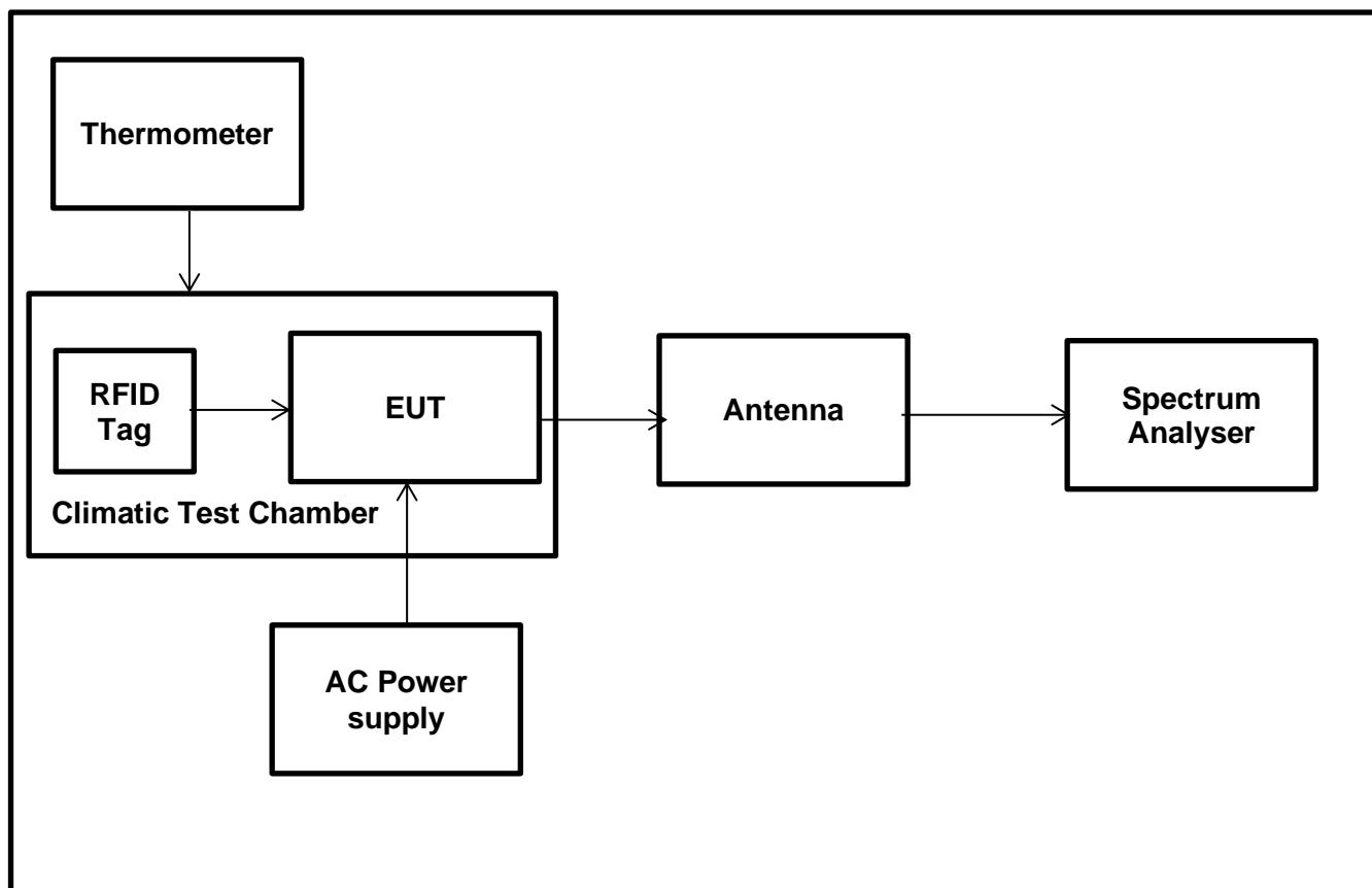
**Transmitter Frequency Stability (Temperature & Voltage Variation) (continued)****Results: AC-DC Power supply / RFID 13.56 MHz / Temperature Variations**
