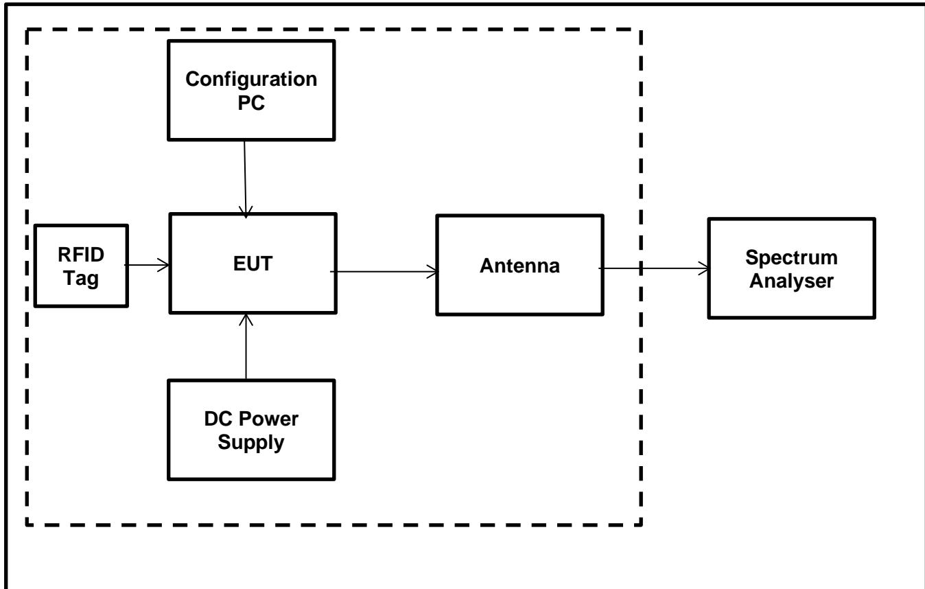
**Transmitter 20 dB Bandwidth (continued)****Results: AC-DC Power Supply / RFID 13.56 MHz**
