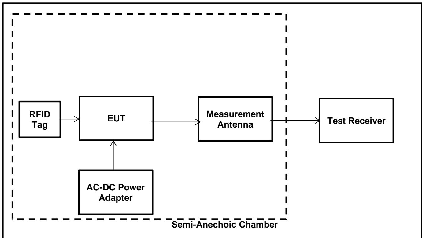
**Transmitter Fundamental Field Strength(continued)****Results: AC-DC Power supply / RFID 13.56 MHz**
