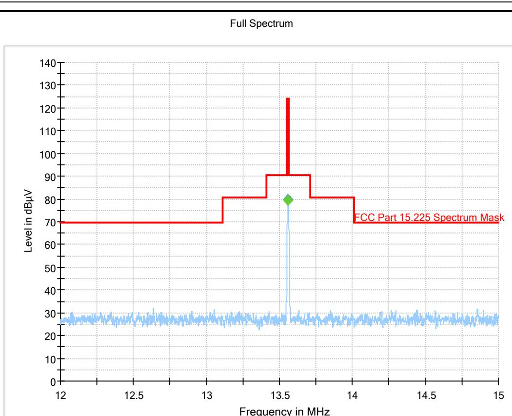
Fundamental field strength and spectrum mask / measured at 3 metres extrapolated to 30 metres / measured in a semi-anechoic chamber
