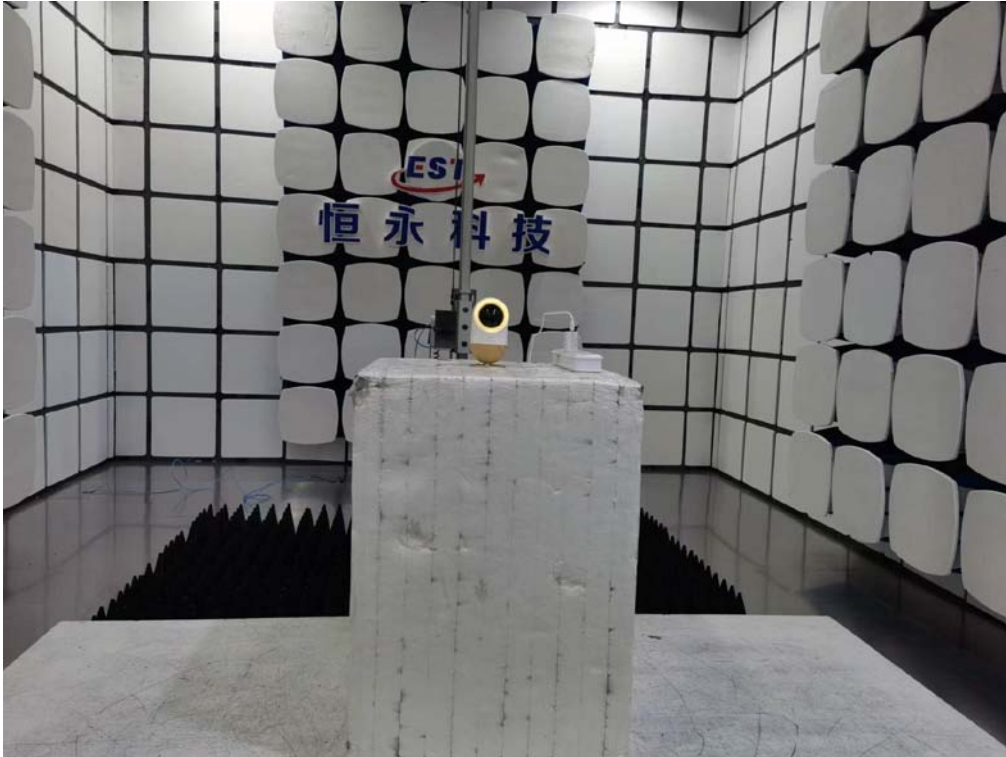
Radiated emission test: Above 1GHz
