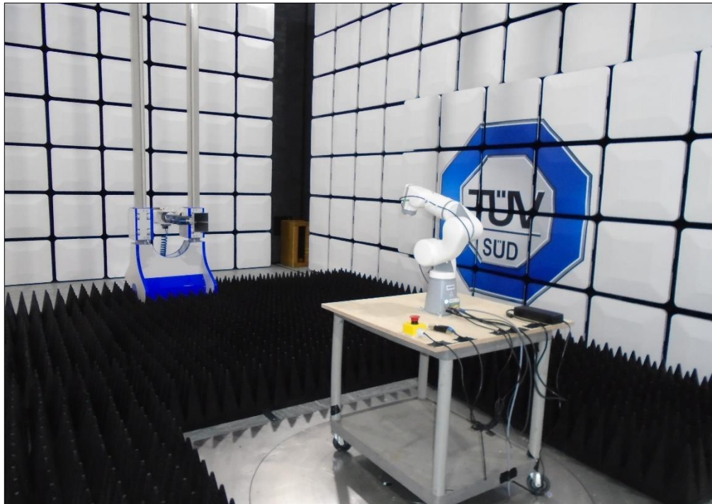
Figure 8 - Test Setup - 1 GHz to 18 GHz
