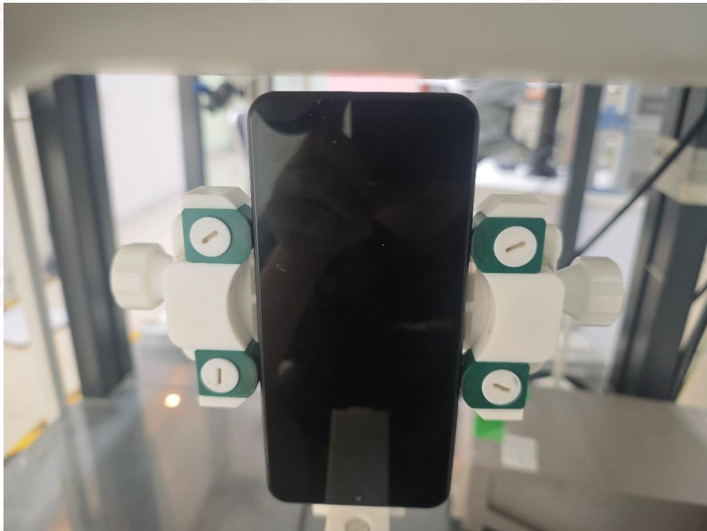
Body Top side(separation distance is 5mm)
