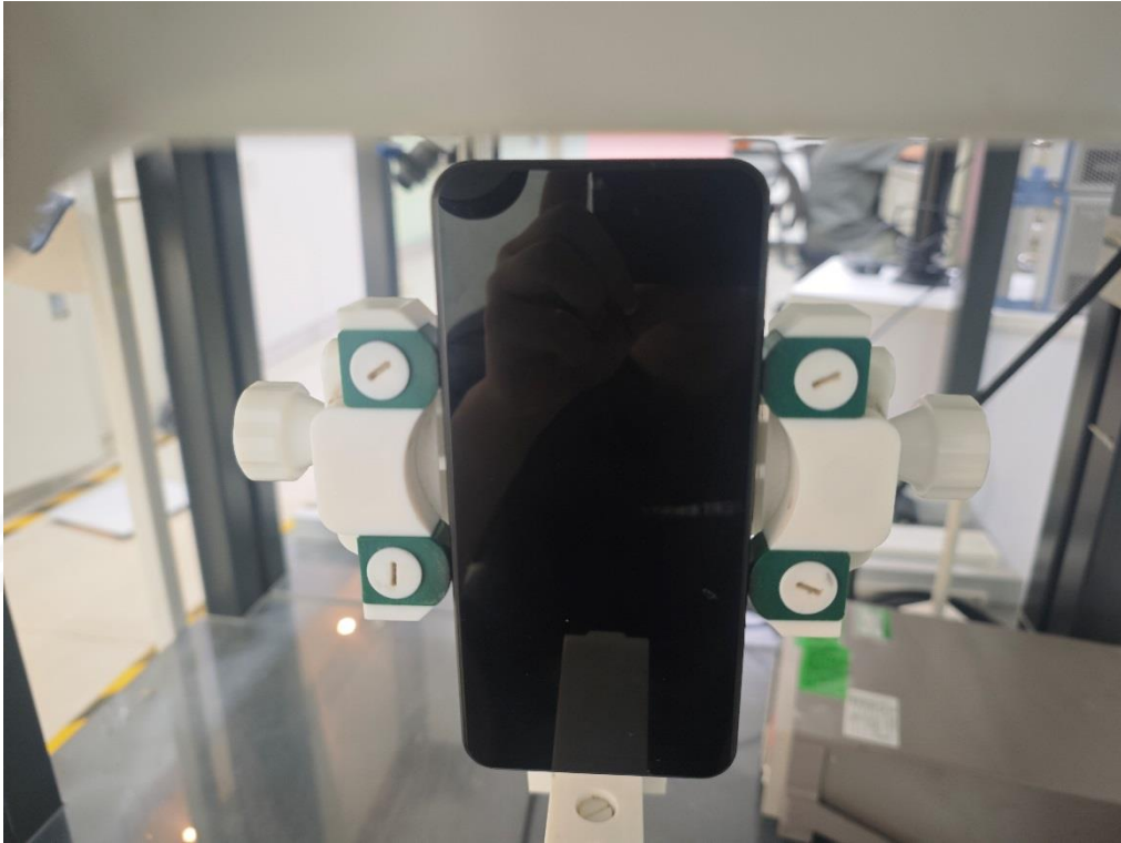
Body Bottom side(separation distance is 5mm)
