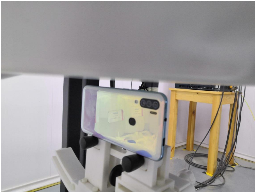
10mm body-worn Right Side Setup Photo (hotspot)
