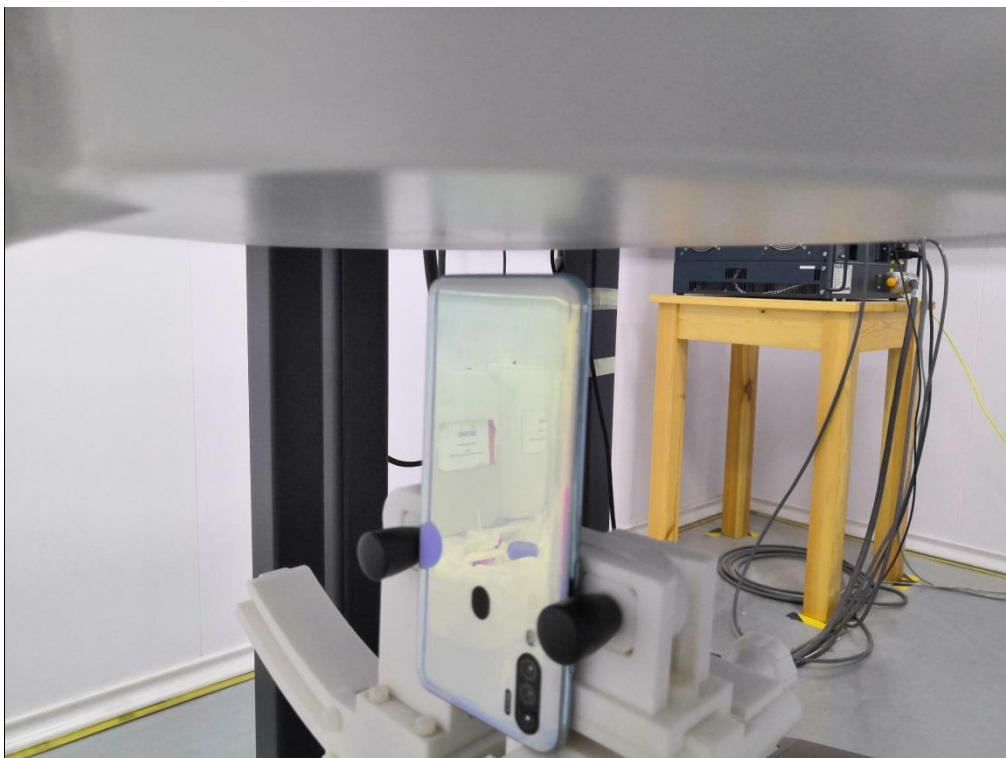
10mm body-worn Bottom Side Setup Photo (hotspot)
