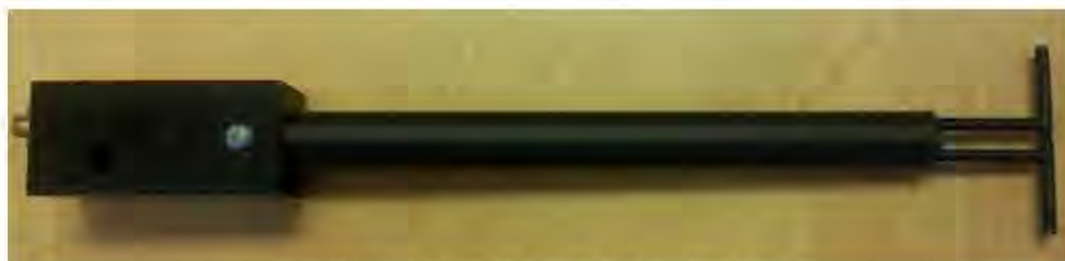
Figure 1 – MVG COMOSAR Validation Dipole
