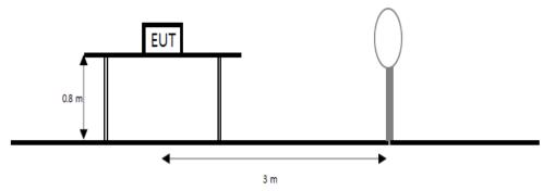
The diagram below shows the test setup that is utilized to make the measurements for emission from 30 Mbz to 1 GHz emissions.
