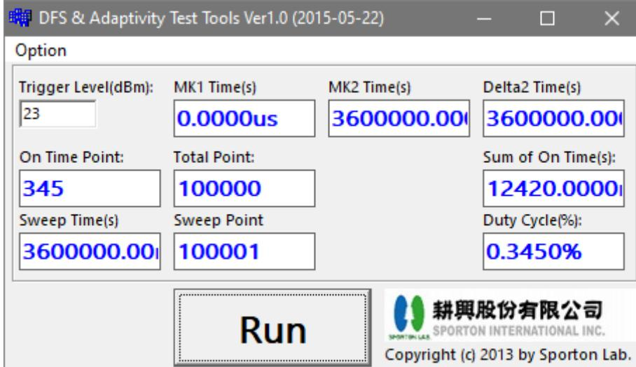
The sum of On Time (aggregated time from marker 1 to 2): 12.42s < 20s, Pass.
