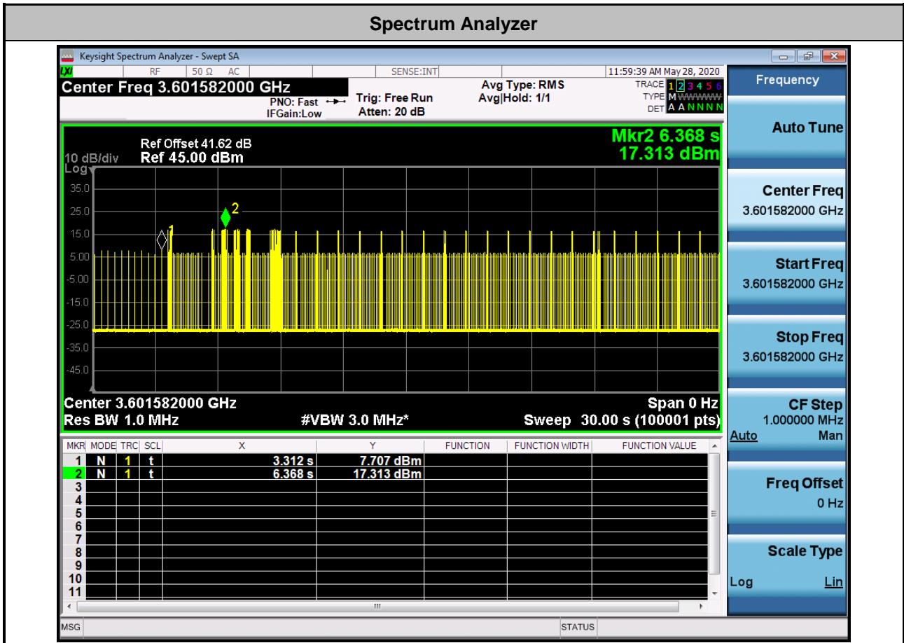
Note : The Ref Offset 41.62 dB includes the antenna gain 13 dBi and cable path loss 28.62 dB.
