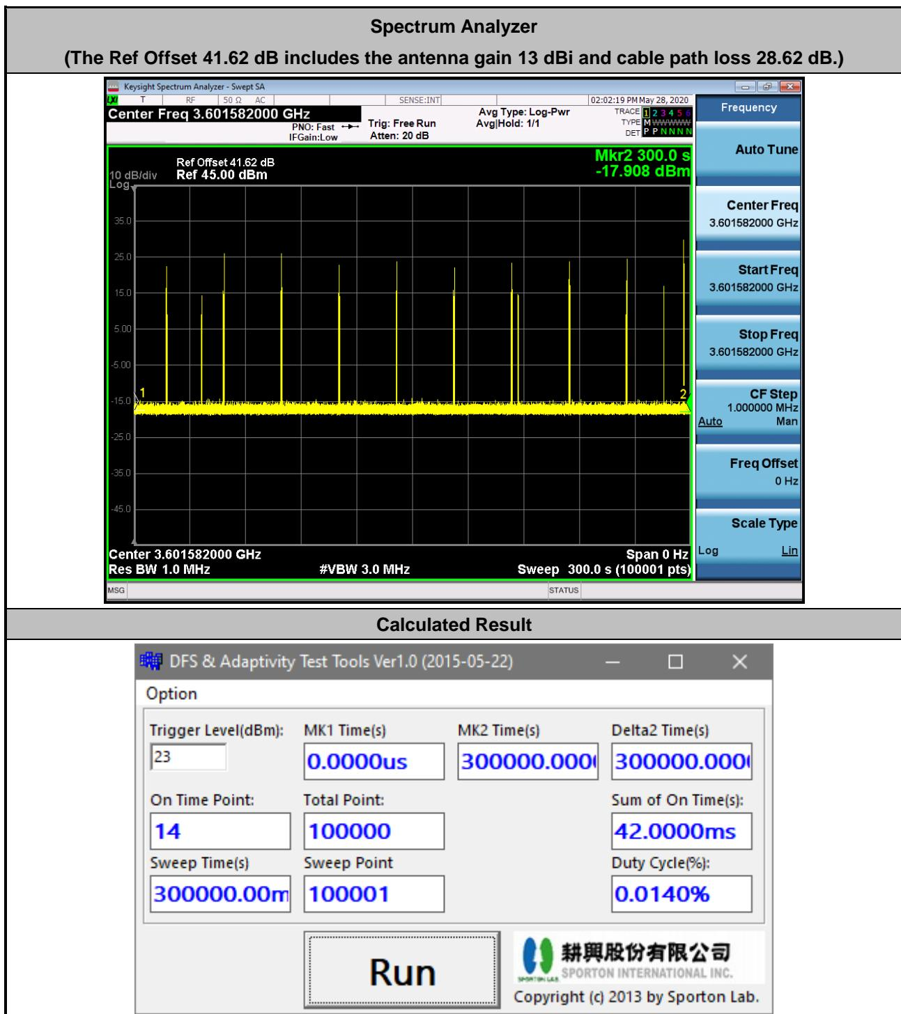
The sum of On Time (aggregated time from marker 1 to 2): 42ms < 10s, Pass.
