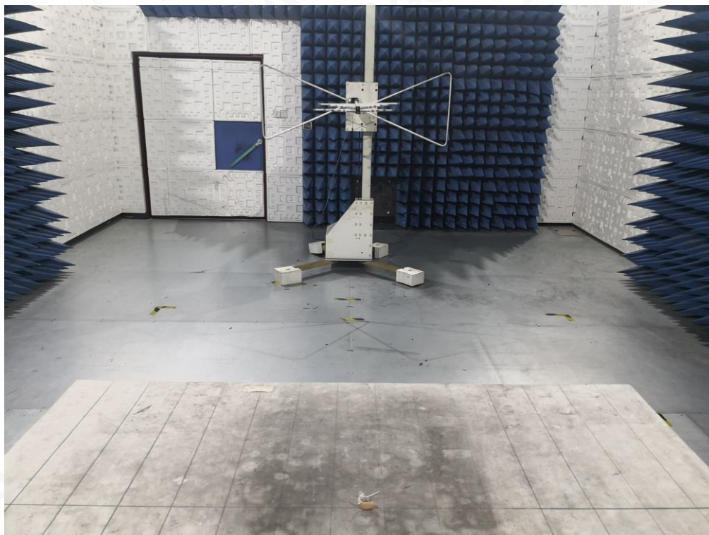
RADIATED EMISSION TEST SETUP ABOVE 1GHZ
