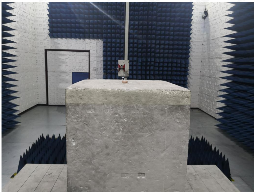
RADIATED EMISSION TEST SETUP ABOVE 1GHZ
