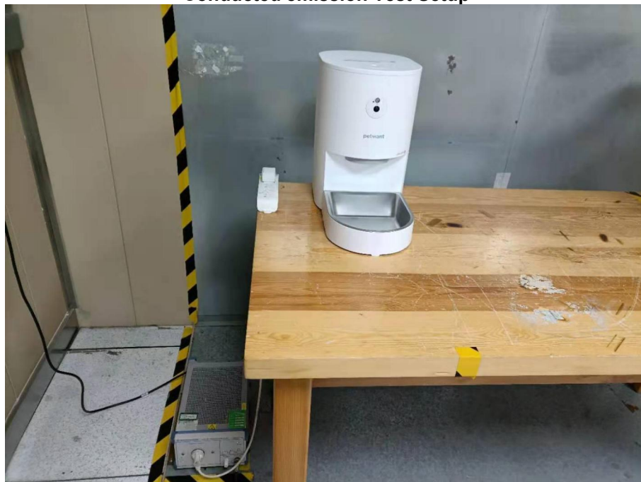
Conducted emission Test Setup
