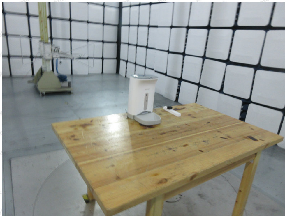
Photo of Radiation Emission Test
