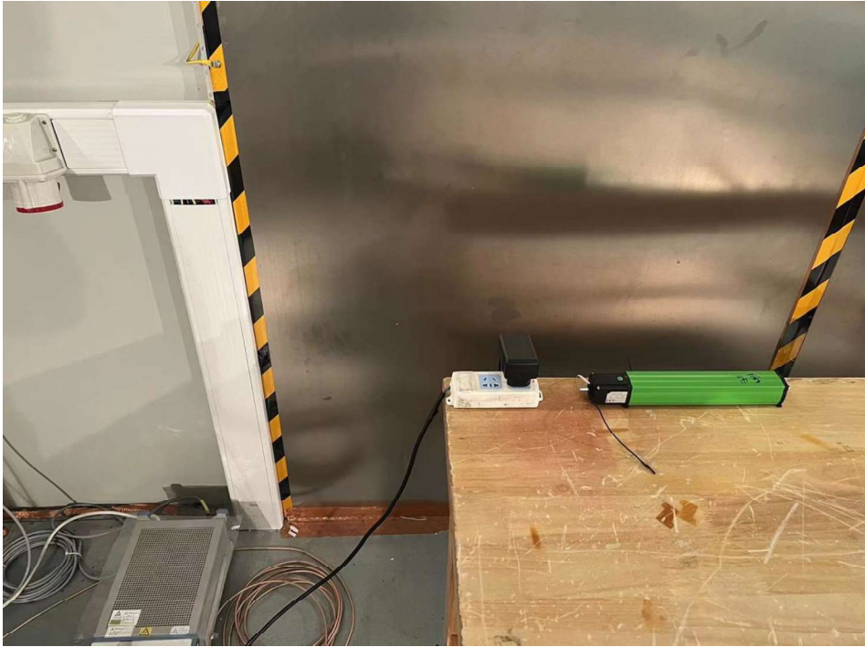
Test Set-up: Conducted emission 150KHz-30MHz
