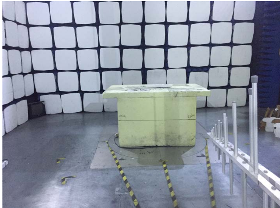
Radiation Emission Test Setup (30MHz to 1GHz)
