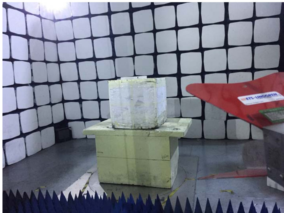
Radiation Emission Test Setup (1GHz to 18GHz)
