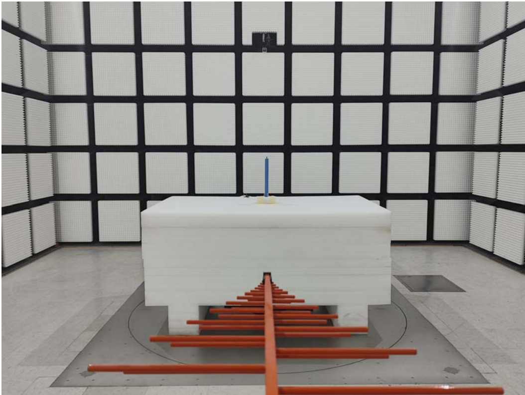
Radiated Emission Above 1GHz View
